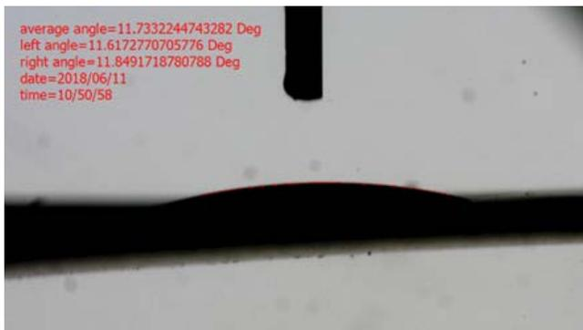
Fig. 4. Contact angle results of the co-polymerized GO.
