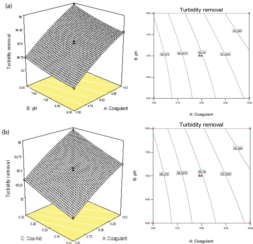
Fig. 4. Two and three dimensional contour plots showing the combined effects of (a) aluminum sulfate dosage and pH, and (b) aluminum sulfate and LT27 dosage on turbidity removal.
