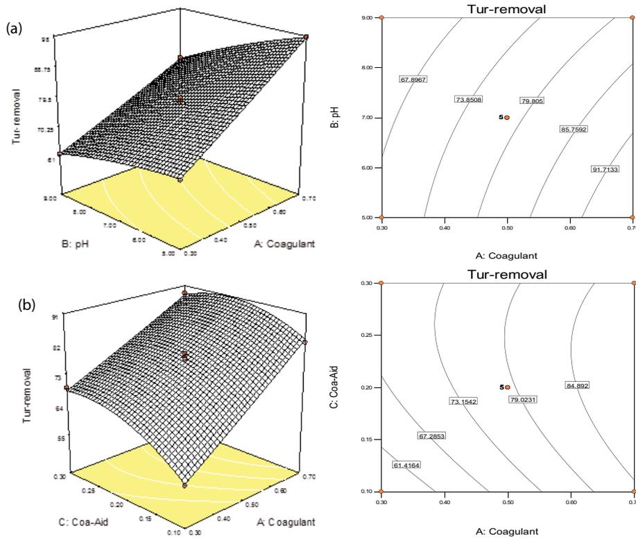
Fig. 5. Two and three dimensional contour plots showing the combined effects of (a) ferric chloride dosage and pH, and (b) ferric chloride and LT25 dosages on turbidity removal.
