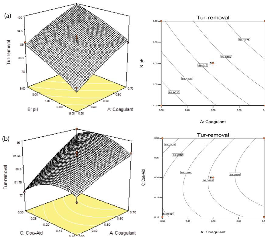
Fig. 6. Two- and three-dimensional contour plots showing the combined effects of (a) ferric chloride dosage and pH, and (b) ferric chloride and LT27 dosages on turbidity removal.
