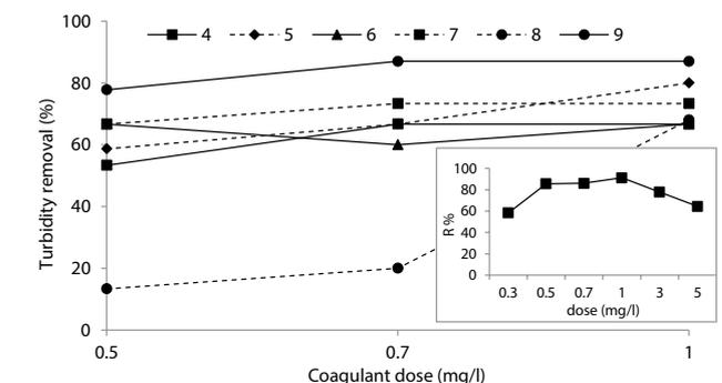
Fig. 2. Effect of the applied ferric chloride dosage and pH on turbidity removal.
