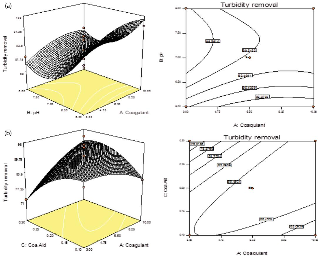
Fig. 3. Two and three dimensional contour plots showing the combined effects of (a) aluminum sulfate dosage and pH, and (b) aluminum sulfate and LT25 dosages on turbidity removal.
