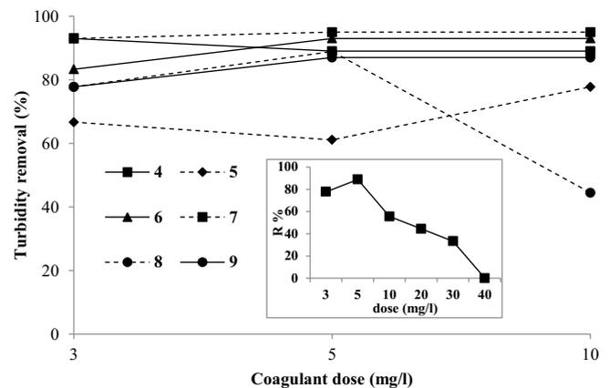
Fig. 1. Effect of aluminum sulfate dosage and pH on turbidity removal.
