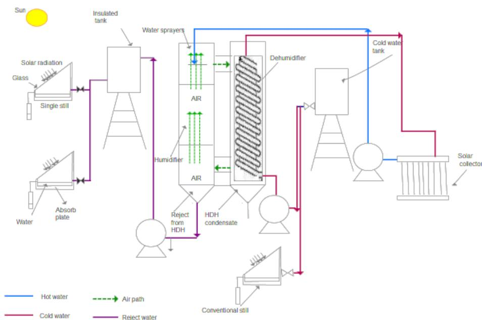
Fig. 7. HDH and solar stills hybrid system.
