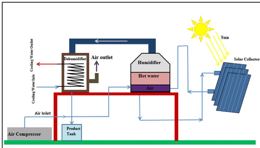
Fig. 11. HDH schematic diagram.
