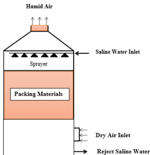
Fig. 4. Schematic diagram of packed bed humidifier.
