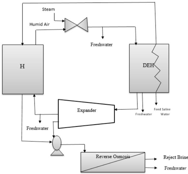
Fig. 14. Schematic diagram of HDH-TVC-RO desalination system.
