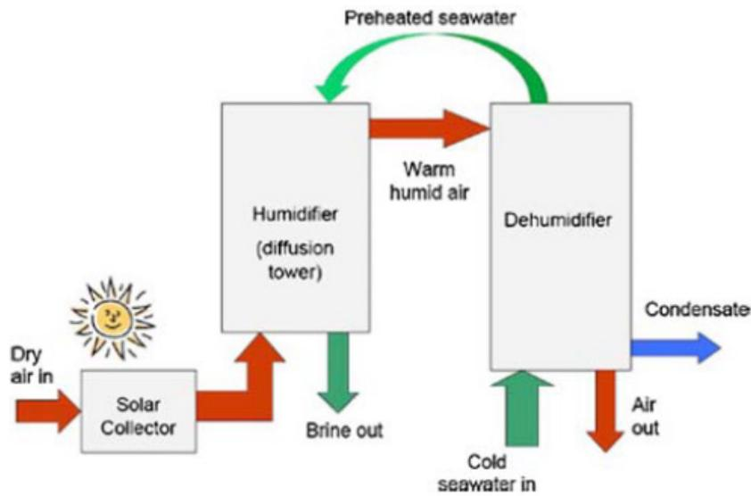
Fig. 3. Humidification-dehumidification cycle [4].
