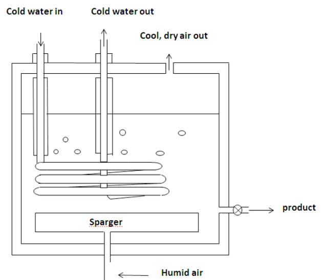
Fig. 12. Schematic diagram of the experimental bubble column dehumidifier.
