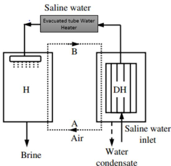
Fig. 5. Schematic of water heated HDH system [4].
