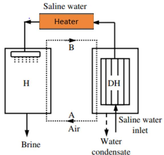
Fig. 6. Scheme of a HD desalination unit using spray humidifier [4].
