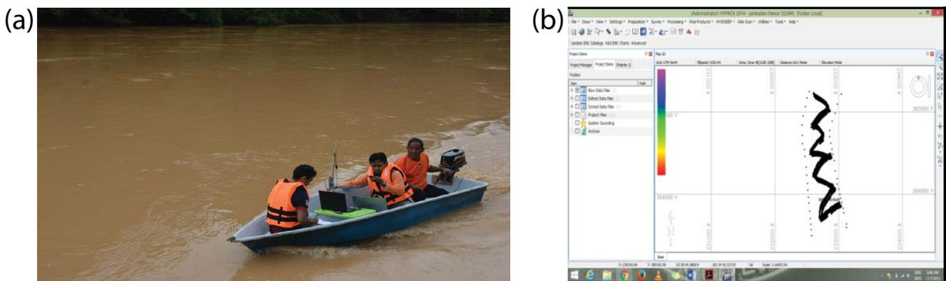
Fig. 5. (a) Bathymetric data sampling at Pahang River Basin, and (b) Surfer 8 application method illustration.
