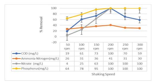
Fig. 1. COD, ammonia nitrogen, nitrate and phosphorus removal at 50, 100, 150 and 200 shaking speed.
