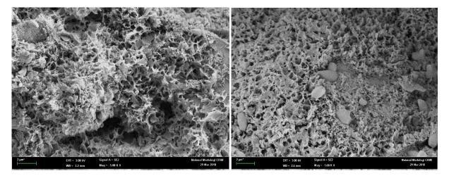
Fig. 5. Composite POFA before adsorption (a) and after adsorption (b).
