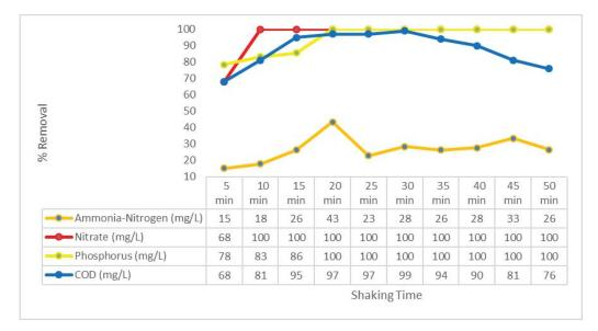
Fig. 2. COD, ammonia nitrogen, nitrate and phosphorus removals at 5, 10, 15, 20, 25, 30, 35, 40, 45 and 50 min shaking time.
