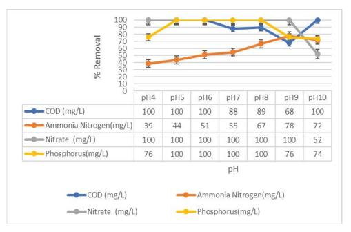
Fig. 3. COD, ammonia nitrogen, nitrate and phosphorus removals at pH, 4, 5, 6, 7, 8, 9 and 10.
