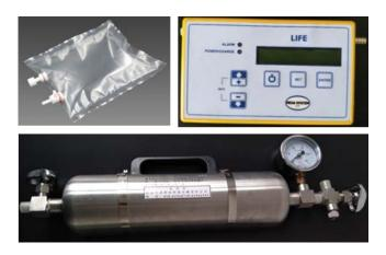
Fig. 2. Tedlar gas sample bags and gas sampler.
