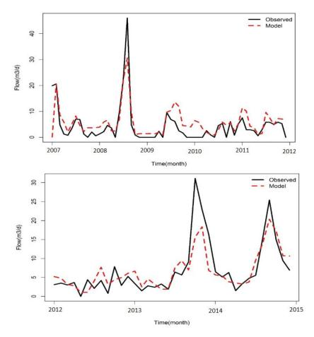
Fig. 3. Observed and simulated hydrographs for location of Jiyunhe for calibration (top) and validation (bottom).
