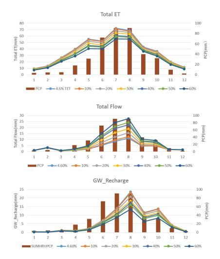
Fig. 8. Effect of impervious cover on total ET, total flow, and groundwater levels at average monthly scale.
