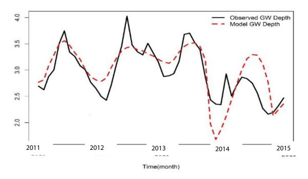
Fig. 4. Observed and simulated groundwater (GW) levels for location of Wuqing District for validation period.
