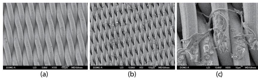
Fig. 6. Structure of wire-mesh with pore size 30  $\mu\text{m}$ : (a) SEM image of clean wire-mesh (100 $\times$ ), (b) SEM image of filtration wire-mesh (50 $\times$ ), and (c) SEM image of filtration wire-mesh (300 $\times$ ).
