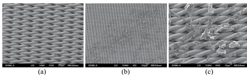
Fig. 4. Structure of wire-mesh with pore size 10  $\mu\text{m}$ : (a) SEM image of clean wire-mesh (100 $\times$ ), (b) SEM image of filtration wire-mesh (50 $\times$ ), and (c) SEM image of filtration wire-mesh (300 $\times$ ).
