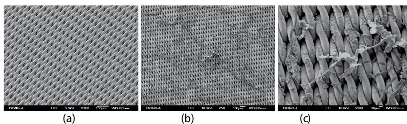
Fig. 3. Structure of wire-mesh with pore size 5  $\mu\text{m}$ : (a) SEM image of clean wire-mesh (100 $\times$ ), (b) SEM image of filtration wire-mesh (50 $\times$ ), and (c) SEM image of filtration wire-mesh (300 $\times$ ).
