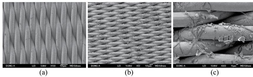
Fig. 5. Structure of wire-mesh with pore size 15  $\mu\text{m}$ : (a) SEM image of clean wire-mesh (100 $\times$ ), (b) SEM image of filtration wire-mesh (50 $\times$ ), and (c) SEM image of filtration wire-mesh (300 $\times$ ).
