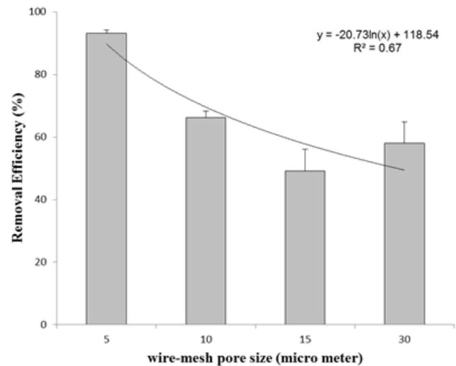
Fig. 1. Single layer wire-mesh removal efficiencies.
