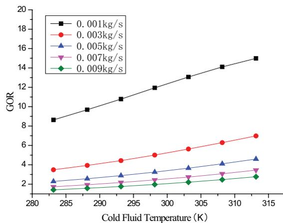
Fig. 7. Effect of cold fluid temperature and flow rate on GOR (concentration 0.62mol/kg, model height 1m, air gap width 5 mm, hot fluid temperature 353.15 K).
