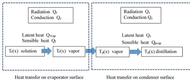
Fig. 4. Diagram of heat transfer in air-gap.
