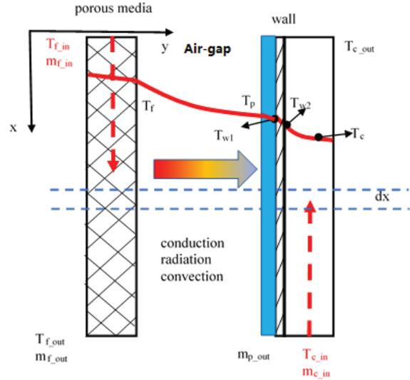
Fig. 2. Air-gap desalination device model.
