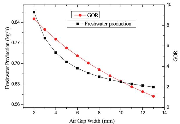
Fig. 10. Effect of air-gap width on freshwater yield and GOR (flow rate 0.003 kg/s, model height 1m, concentration 0.62mol/kg, hot fluid temperature 353.15 K, cold fluid temperature 293.15 K).
