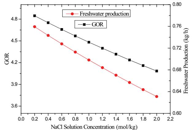
Fig. 9. Effect of NaCl solution concentration on freshwater yield and GOR (flow rate 0.003kg/s, model height 1m, air-gap width 5 mm, hot fluid temperature 353.15 K, cold fluid temperature 293.15 K).
