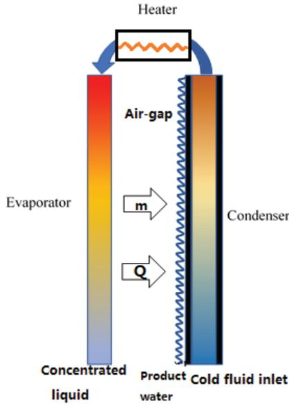
Fig. 1. Schematic diagram of working medium flow process in AGDD device.
