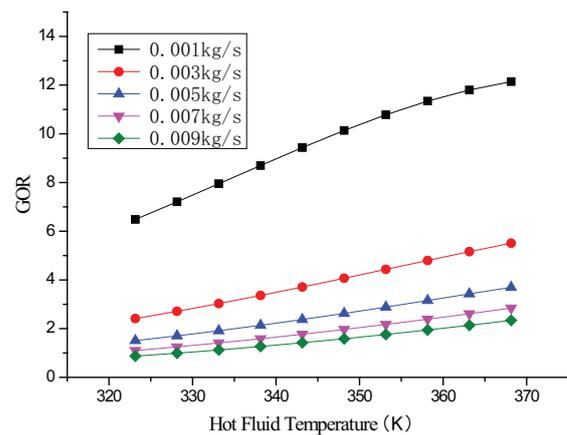
Fig. 6. Effect of hot fluid temperature and flow rate on GOR (concentration 0.62 mol/kg, model height 1m, air-gap width 5 mm, cold fluid temperature 293.15 K).
