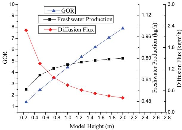
Fig. 11. Effect of model height on yield, GOR, and diffusivity (flow rate 0.003 kg/s, air gap width 5 mm, concentration 0.62 mol/kg, hot fluid temperature 353.15 K, cold fluid temperature 293.15 K).
