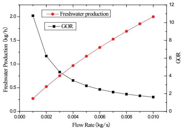
Fig. 8. Effect of flow rate on freshwater yield and GOR (concentration 0.62mol/kg, model height 1m, air-gap width 5 mm, hot fluid temperature 353.15 K, cold fluid temperature 293.15 K).
