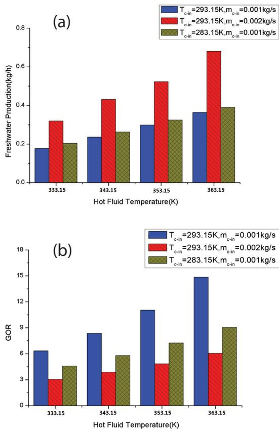
Fig. 12. Effect of cold fluid temperature, hot fluid temperature and flow rate on GOR and freshwater production (concentration 0.62 mol/kg, model height 1 m, air-gap width 5 mm).
