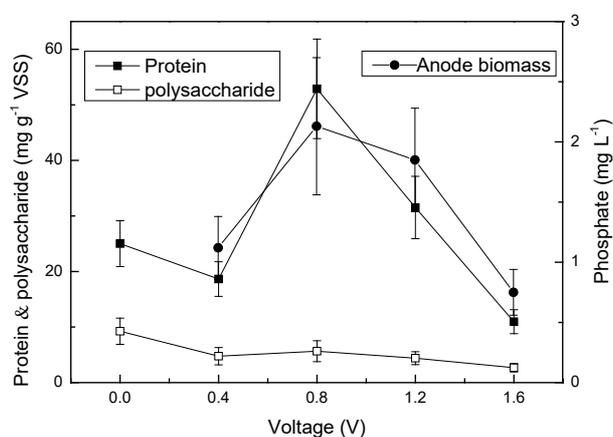
Fig. 8. Effect of applied voltage on anode biomass and EPS contents of the biofilms after start-up.
