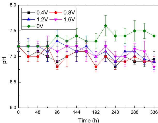
Fig. 4. The pH of MEC reaction solution varied with time under different external voltages.
