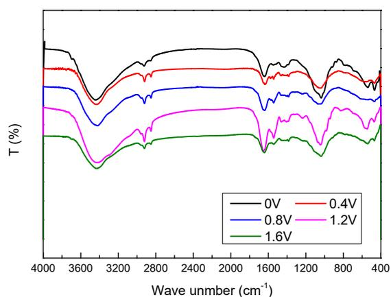
Fig. 9. FT-IR spectra of EPS in anode biofilms at different applied voltages.
