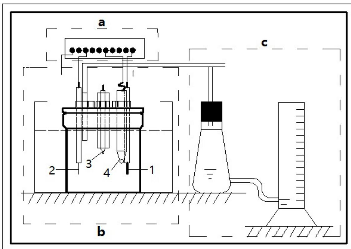
Fig. 1. Single chamber MEC shown with online recorder (a), fermentation chamber (b), gas collection unit (c), anode electrode (1), cathode electrode (2), pH electrode (4), Ag/AgCl-KCl reference electrode (3).
