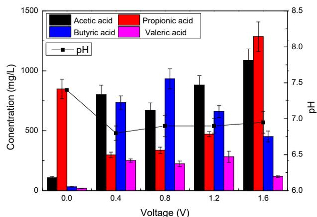
Fig. 5. End-production concentrations and pH variation of MECs with biofilm enriched at different culture voltages.
