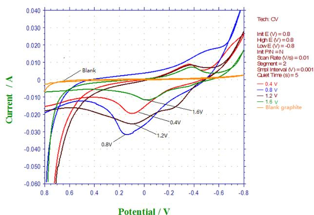
Fig. 6. The cyclic voltammogram obtained for different enrichment voltages.
