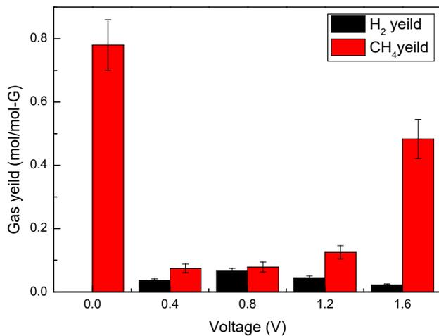
Fig. 3. Hydrogen and methane production under different culture voltages.
