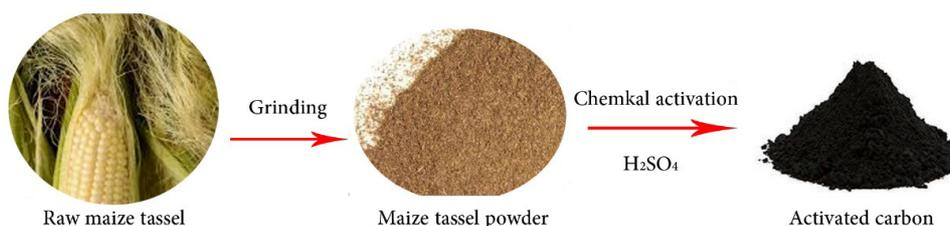
Fig. 1. Schematic representation of the process involved in the derivation of activated carbon from raw maize tassel up to adsorption.
