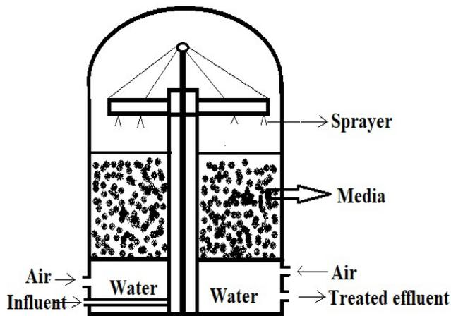
Fig. 2. Schematic representation of trickling filters [17].
