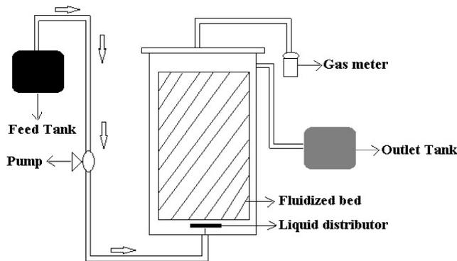
Fig. 10. Schematic representation of anaerobic fluidized bed reactor [105].
