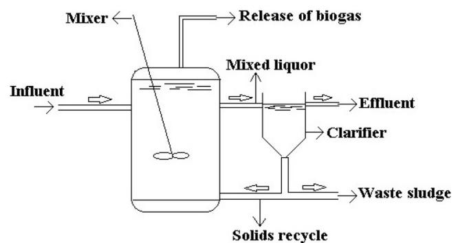
Fig. 9. Schematic representation of anaerobic contact process [14].
