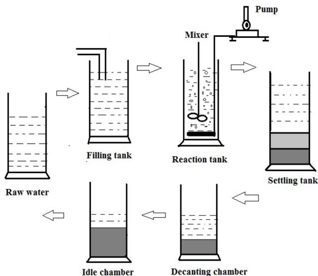
Fig 5. Schematic representation of sequencing batch reactor [17].
