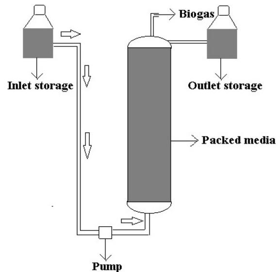
Fig. 11. Schematic representation of anaerobic packed bed reactor [14].
