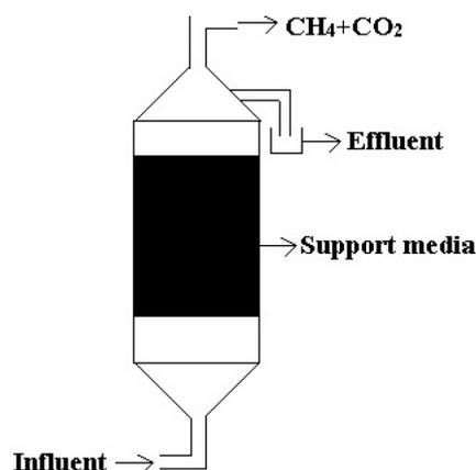
Fig. 6. Diagrammatic representation of anaerobic filters [14].
