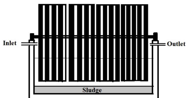
Fig 4. Schematic representation of rotating biological contactors [61].
