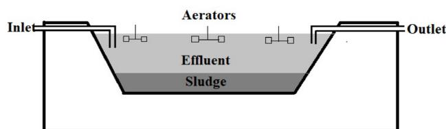
Fig. 1. Schematic representation of aerated lagoons [17].
