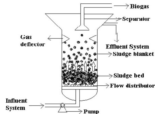
Fig. 7. Schematic representation of up-flow anaerobic sludge blanket reactor (UASB) [85].
