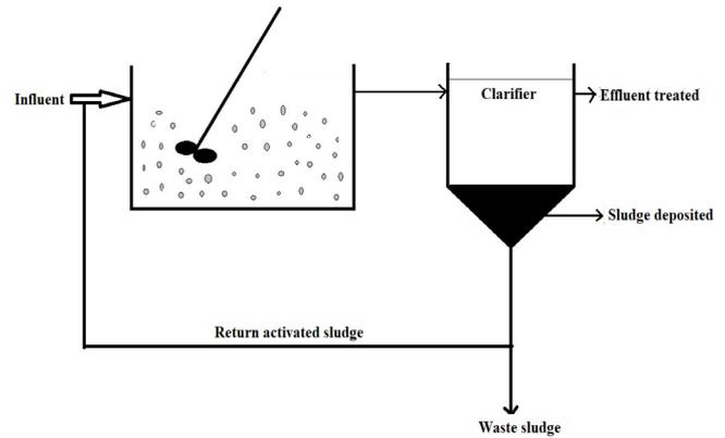
Fig. 3. Diagrammatic representation of activated sludge process [17].
