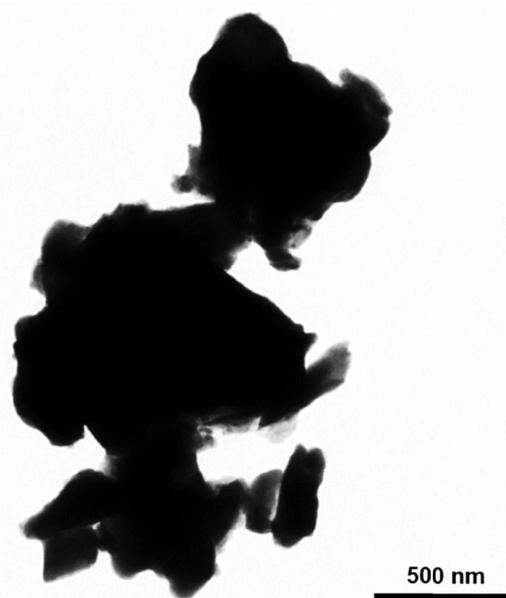
Fig. S1. TEM image of as-received circulating fluidized bed fly ash.
