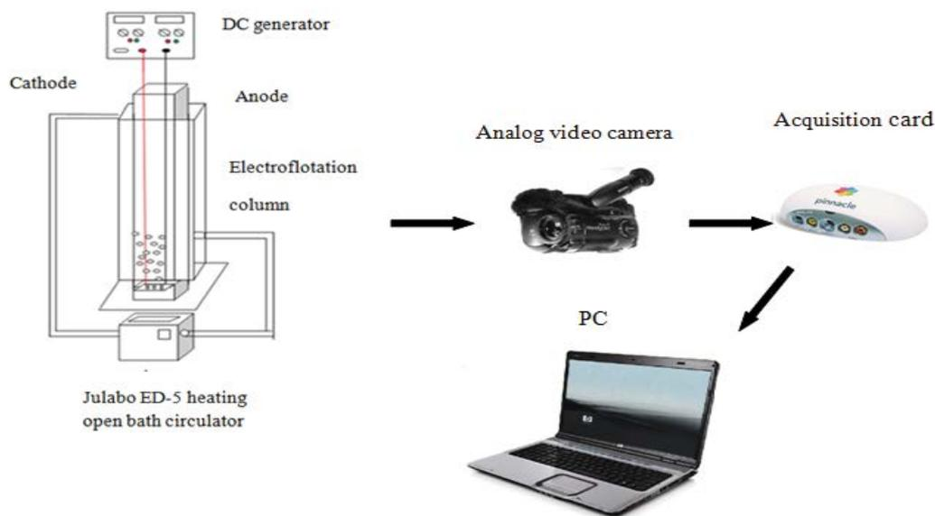
Fig. 1. Schematic diagram of the electroflotation column and equipment used.
