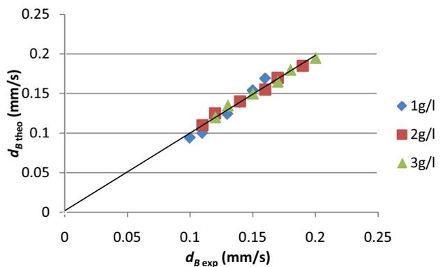
Fig. 6. Comparison between predicted values and experimental values of bubble diameter.
