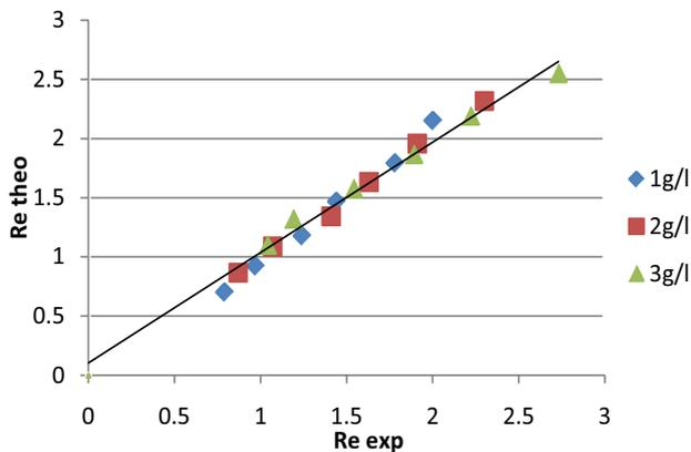
Fig. 8. Comparison of experimental data and predicted values of Reynolds number.
