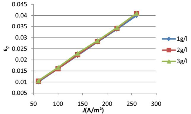
Fig. 5. Effect of current density and oil concentration on gas holdup.
