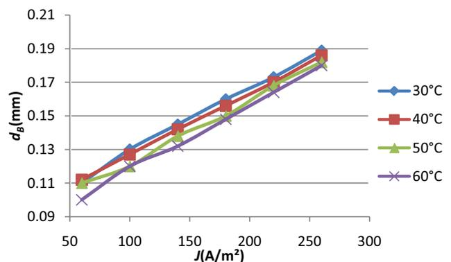
Fig. 9. Effect of temperature on bubble diameter for different oil/water emulsions.
