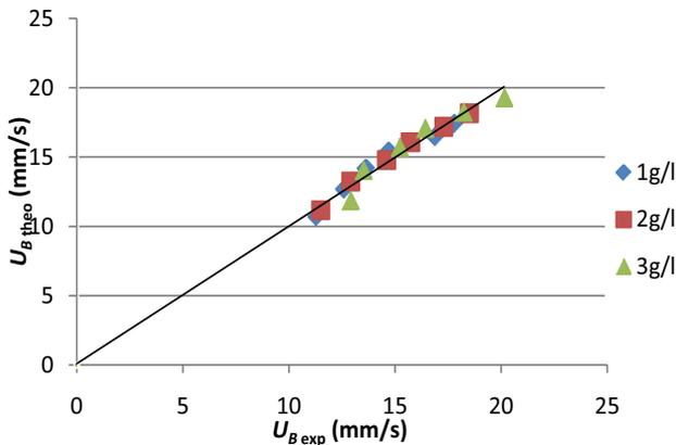
Fig. 7. Comparison of experimental values and predicted values of bubble velocity.
