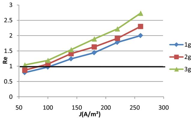
Fig. 4. Effect of current density and oil concentration on Reynolds number.
