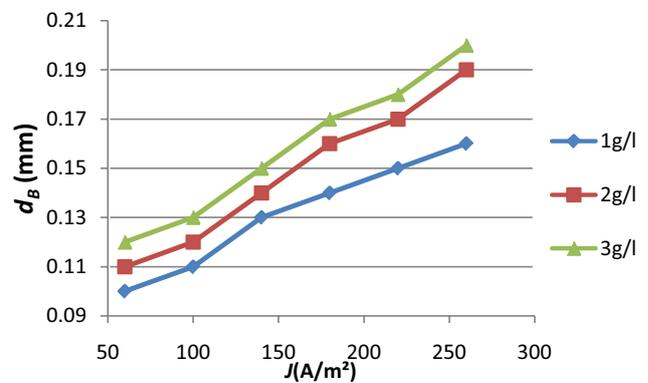
Fig. 2. Effect of current density and oil concentration on bubble diameter.
