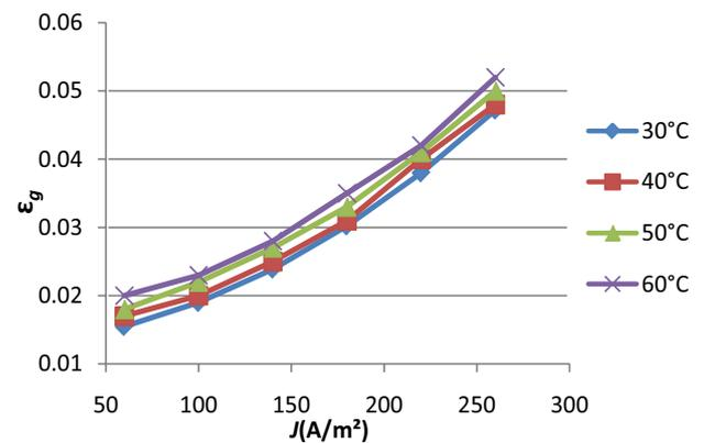
Fig. 12. Effect of temperature on gas holdup for different oil/water emulsions.
