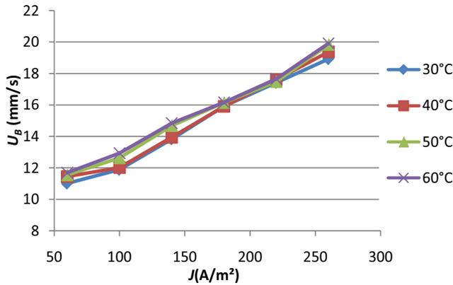
Fig. 10. Effect of temperature on bubble velocity for different oil/water emulsions.
