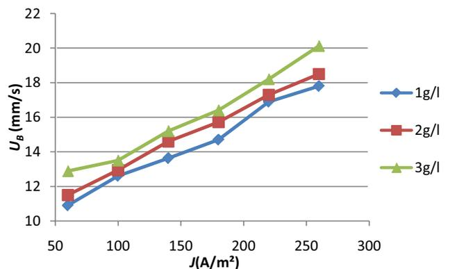
Fig. 3. Effect of current density and oil concentration on bubble velocity.
