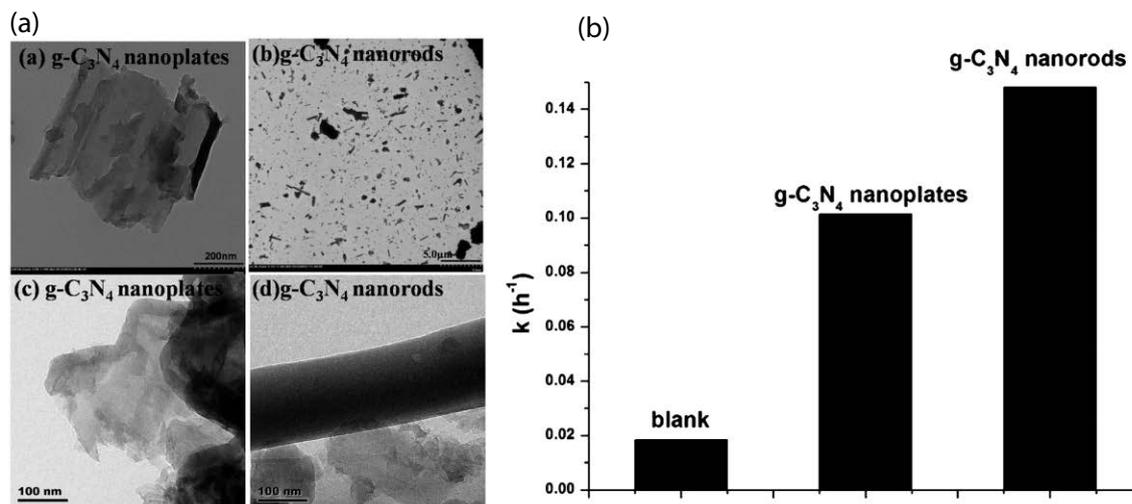
Fig. 2. TEM images of g-C<sub>3</sub>N<sub>4</sub> nanoplates and g-C<sub>3</sub>N<sub>4</sub> nanorods (a); apparent rate constants for MB photodegradation over g-C<sub>3</sub>N<sub>4</sub> nanoplates and g-C<sub>3</sub>N<sub>4</sub> nanorods under visible light and (b). Reprinted with permission from the study of Bai et al. [84]. Copyright © 2013, American Chemical Society.
