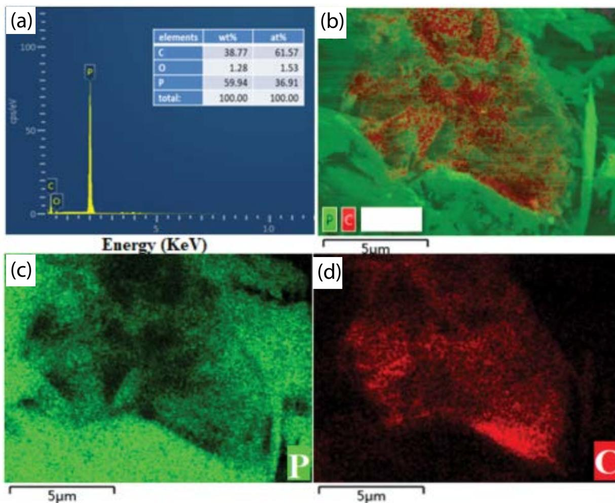
Fig. 6. Images of the synthesized GR-BP hybrid: (a) EDS spectrum of 30% GR-BP hybrid, (b) EDS elemental dot-mapping, (c) P element dot-mapping and (d) C element dot-mapping. Reprinted with permission from the study of Shen et al. [120]. Copyright©2019, Elsevier Publishing Group.
