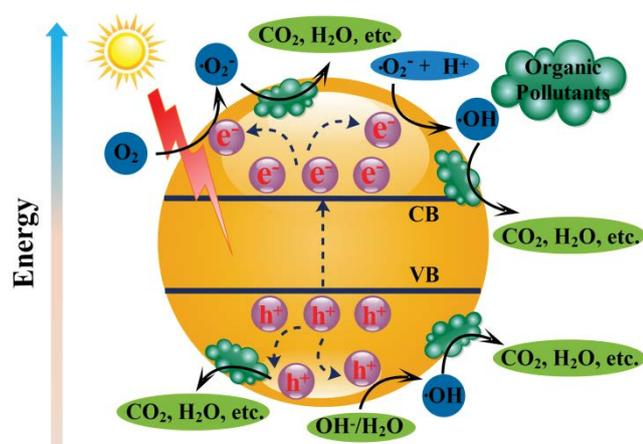
Fig. 1. Possible carrier transfer behaviors and photocatalytic degradation processes of organic pollutants over the semiconductor photocatalyst under the light excitation.
