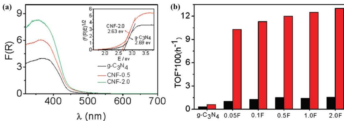
Fig. 3. UV–Vis DRS spectra (a) and optical band gap (inset) of g-C<sub>3</sub>N<sub>4</sub> and CNF-x; catalytic oxidation of benzene using CNF-x (b). Reprinted with permission from the study of Wang et al. [94]. Copyright © 2010, American Chemical Society.
