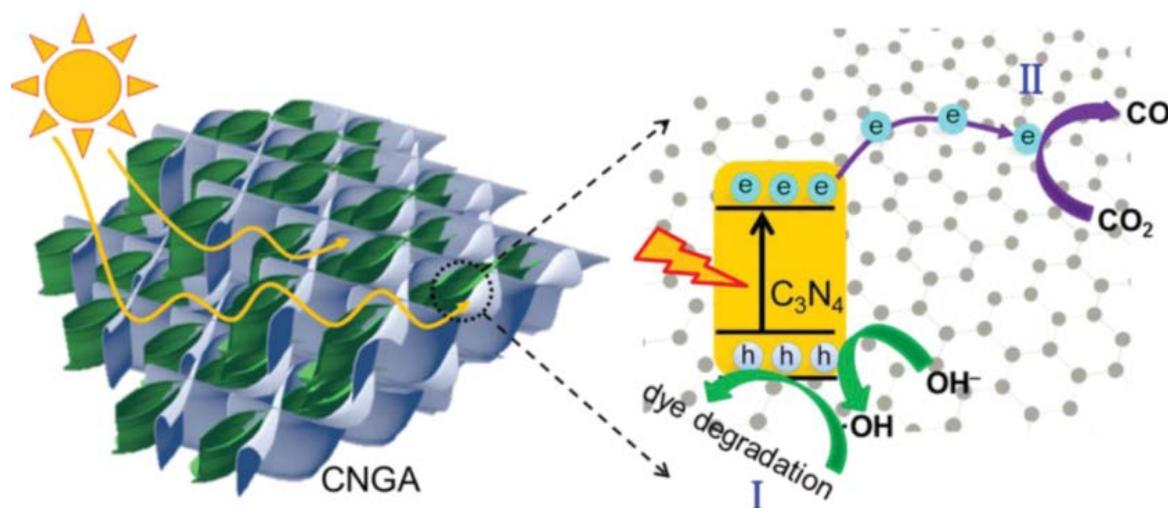
Fig. 4. Schematic diagram for illustrating the photodegradation (I) and photoreduction (II) processes over CNGA under visible-light irradiation. Reprinted with permission from the study of Fang et al. [101]. Copyright© 2015, American Chemical Society.
