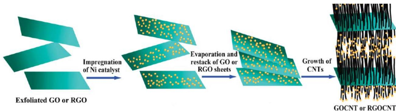
Fig. 5. Experimental steps of pillaring GO and RGO platelets with CNTs. Reprinted with permission from the study of Tsang et al. [111]. Copyright© 2010, American Chemical Society.
