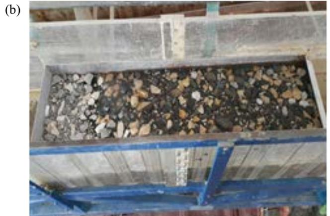
Fig. 2. Porous weir filled with limestone (a) schematic and (b) photo.
