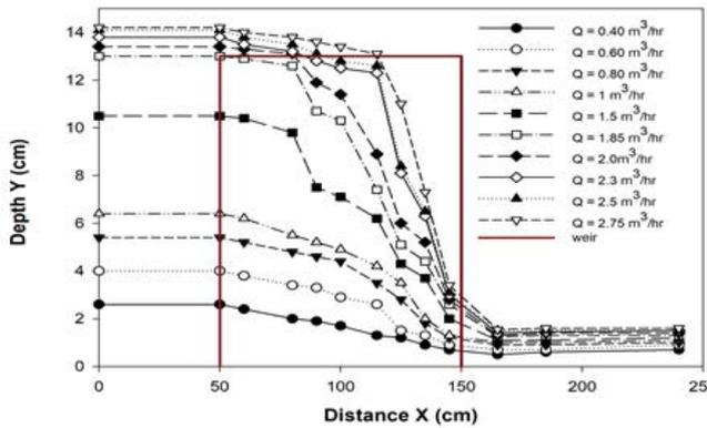
Fig. 7. Experimental water surface profile.
