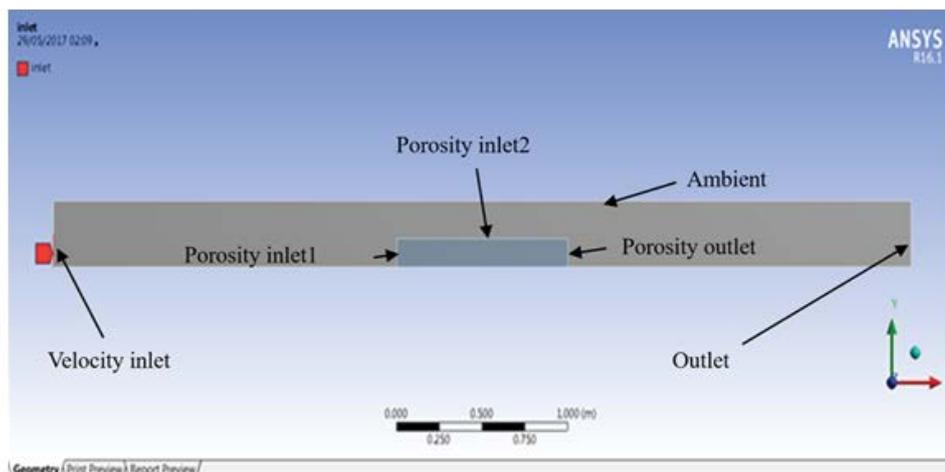
Fig. 6. Boundary conditions for numerical simulation of weirs.
