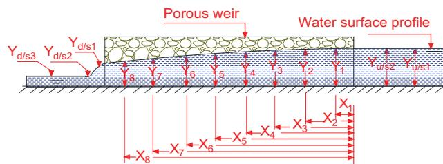
Fig. 4. Schematic showing the locations of distances and depths measured.
