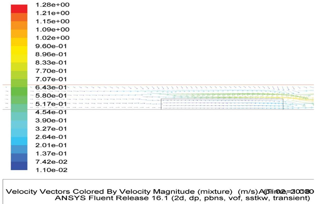
Fig. 15. Velocity vectors for  $Q = 2.75 \text{ m}^3 \text{ h}^{-1}$ .
