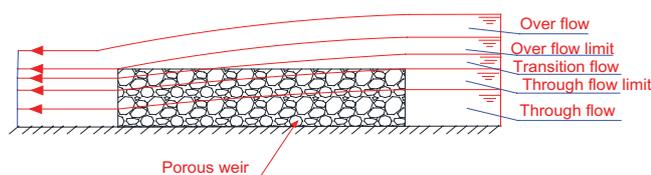
Fig. 5. Five types of flow through and over limestone porous weir.
