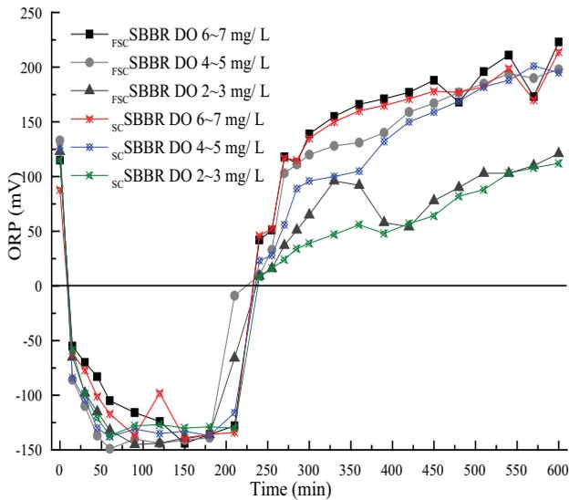
Fig. 6. Changes in ORP in  $f_{SC}$ -SBBR and  $s_{SC}$ -SBBR under different DO conditions.
