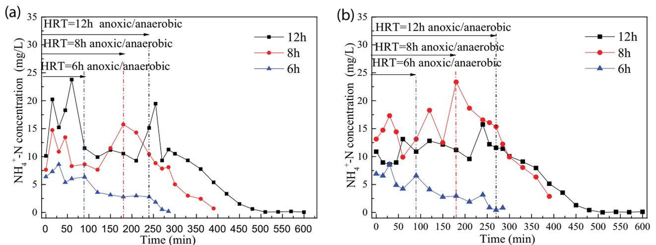
Fig. 8. Periodic variation of ammonia nitrogen contents in the supernatants of  $f_{sc}$ -SBBR and  $sc$ -SBBR at different HRTs.
