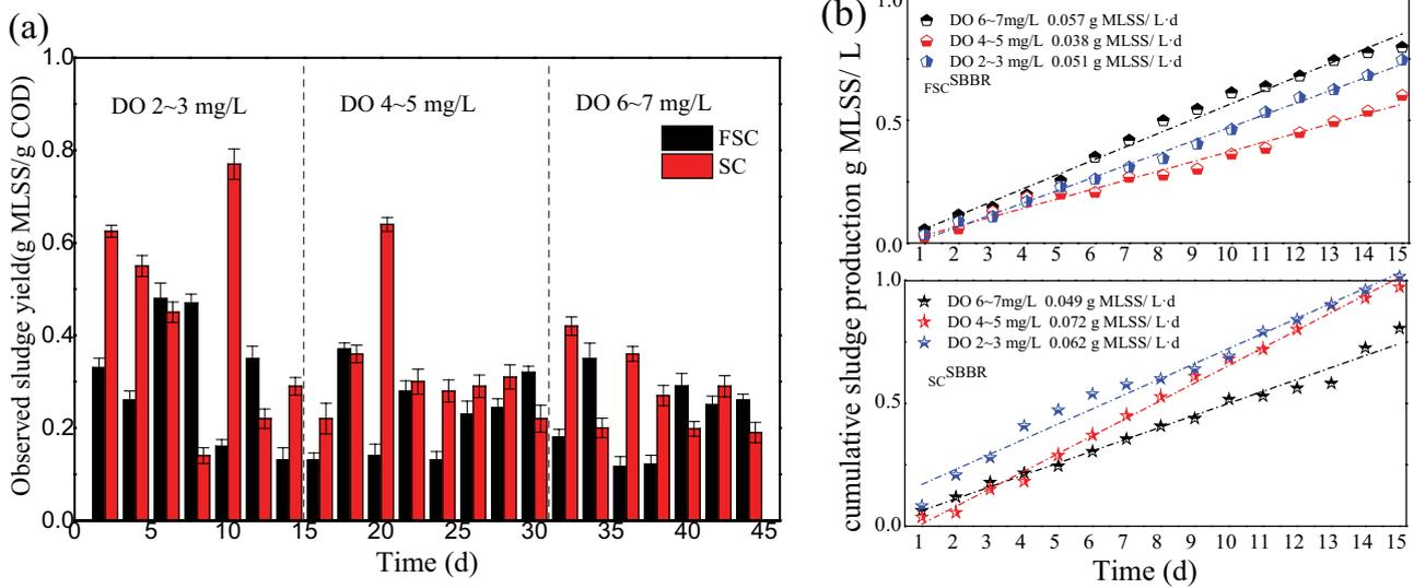
Fig. 5. Daily  $Y_{obs}$  (a) and cumulative sludge production (b) of  $f_{SC}$ -SBBR and  $s_{SC}$ -SBBR at different DO concentrations.
