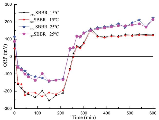
Fig. 3. Changes in ORP in  $f_{sc}$ SBBR and  $s_{c}$ SBBR at different temperatures.
