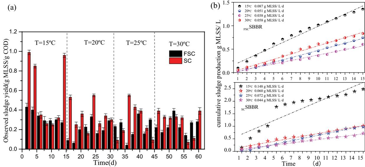
Fig. 2. Daily  $Y_{obs}$  (a) and cumulative sludge production and (b) of  $f_{sc}$ SBBR and  $s_{c}$ SBBR at different temperatures.
