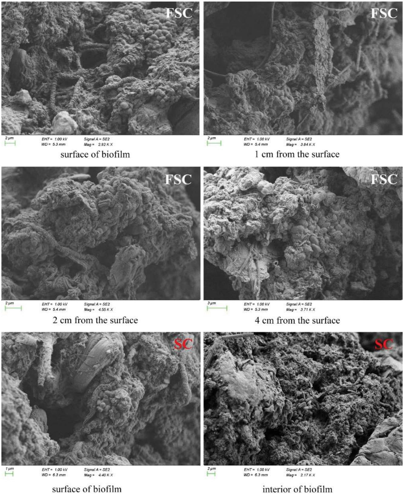
Fig. 9. SEM of biofilms in different regions of (a) <sub>FSC</sub>SBBR and (b) <sub>SC</sub>SBBR (from the surface to the bottom of the carrier).
