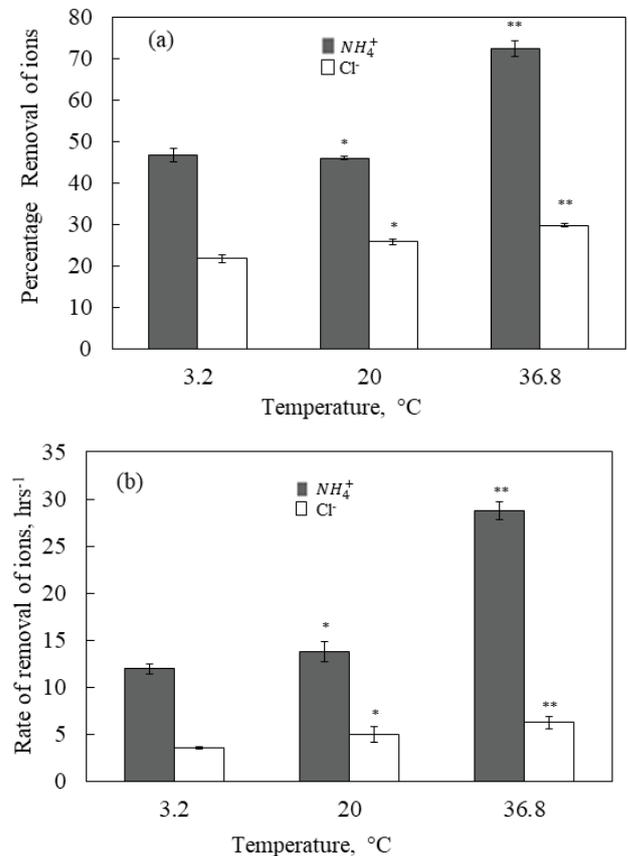
Fig. 5. Effect of temperature on (a) removal percentage and (b) removal rate of  $\text{NH}_4^+$  and  $\text{Cl}^-$  ions after 6 h at 0.1167 A/cm<sup>2</sup> and 14,250 and 20,000 mg/L initial concentrations of  $\text{NH}_4^+$  and  $\text{Cl}^-$  ions, respectively.
