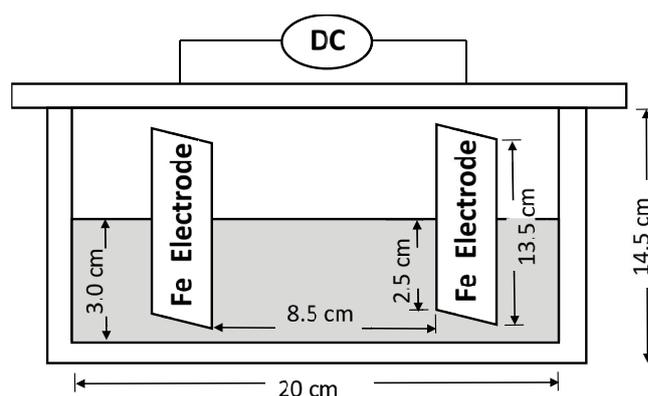
Fig. 1. Schematic diagram of the EC reactor.
