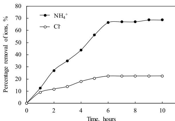
Fig. 2. Removal percentage of  $\text{NH}_4^+$  and  $\text{Cl}^-$  as a function of time at  $30^\circ\text{C}$ ,  $0.167 \text{ A/cm}^2$  current density and initial concentrations of 15,594 and 27,500 mg/L, respectively.
