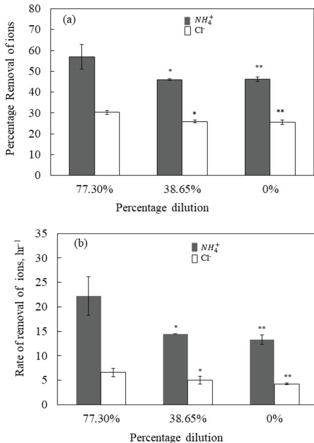
Fig. 4. Effect of initial concentration of  $\text{NH}_4^+$  and  $\text{Cl}^-$  on (a) removal percentage and (b) removal rate after 6 h at 20°C and 0.1167 A/cm<sup>2</sup>. The dilution is considered with respect to the maximum concentration of 17,875 and 32,600 mg/L for  $\text{NH}_4^+$  and  $\text{Cl}^-$ , respectively.
