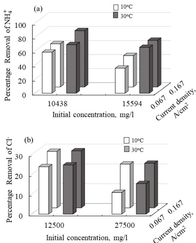
Fig. 6. Effect of current density and initial concentration on removal percentage of (a)  $\text{NH}_4^+$  and (b)  $\text{Cl}^-$  ions after 6 h at 10 and 30°C.
