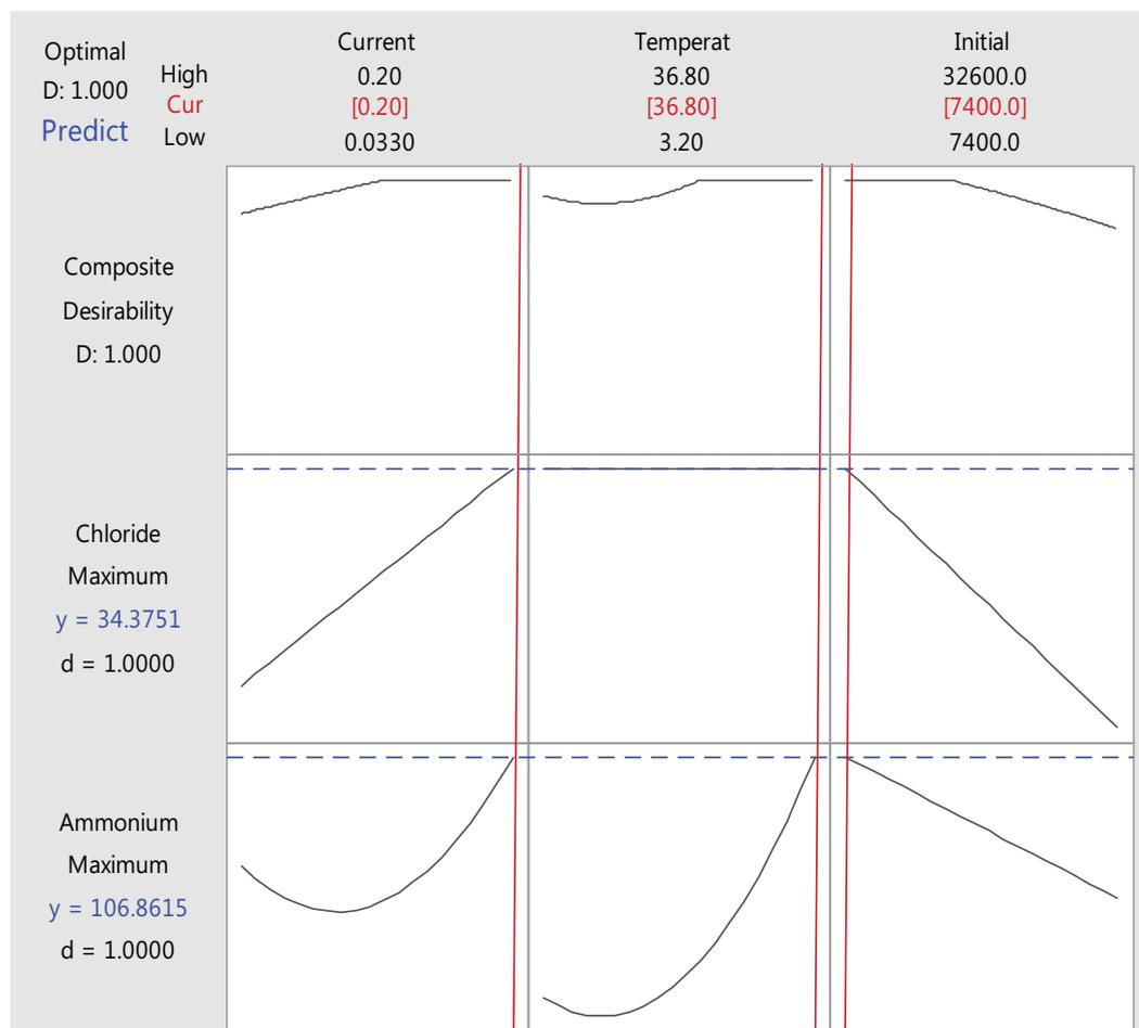
Fig. 7. Optimization results of the effects of current density, temperature and initial concentration for maximum chloride and ammonium removals.
