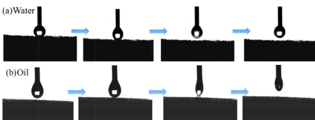
Fig. 5. Wetting behavior of water (a), kerosene (b) droplets on Ota-PDA-PU sponge surface.
