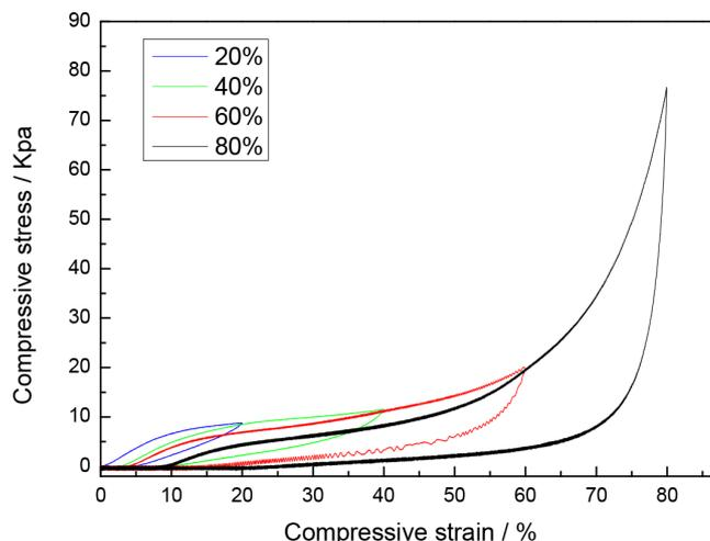
Fig. 3. Loading and unloading compressive stress-strain curves of Ota-PDA-PU sponge at different set strains of 20%, 40%, 60%, and 80%, respectively.
