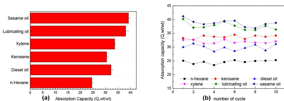
Fig. 7. (a) Oil and organic solvent-absorption capacities of the Ota-PDA-PU sponge. (b) Absorption recyclability of the Ota-PDA-PU sponges for oils and organic solvents.
