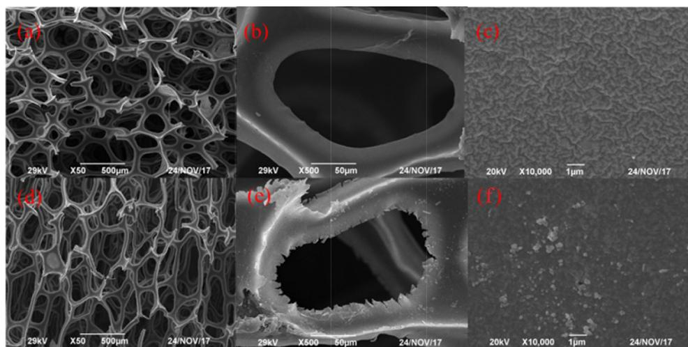
Fig. 1. SEM images with different magnifications for pure PU sponge (a, b and c) and (d, e and f) Ota-PDA-PU sponge.
