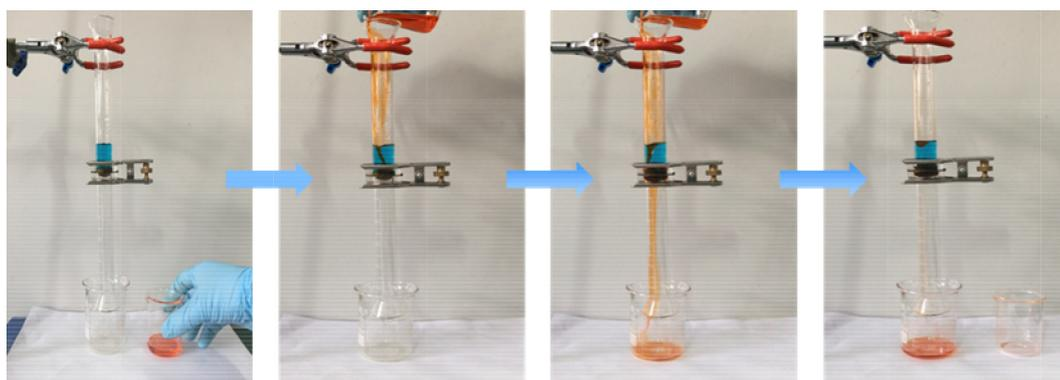
Fig. 8. (a) Oil/water separation studies of the Ota-PDA-PU sponge. For clarity, the tetrachloromethane was dyed by Sudan II and water was dyed by methylene blue.
