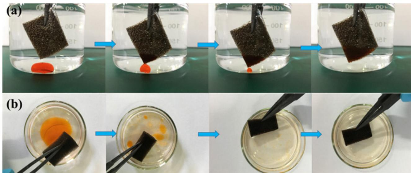
Fig. 6. Snapshots for the process of separating (a) tetrachloromethane and (b) kerosene from water with Ota-PDA-PU sponge, respectively.
