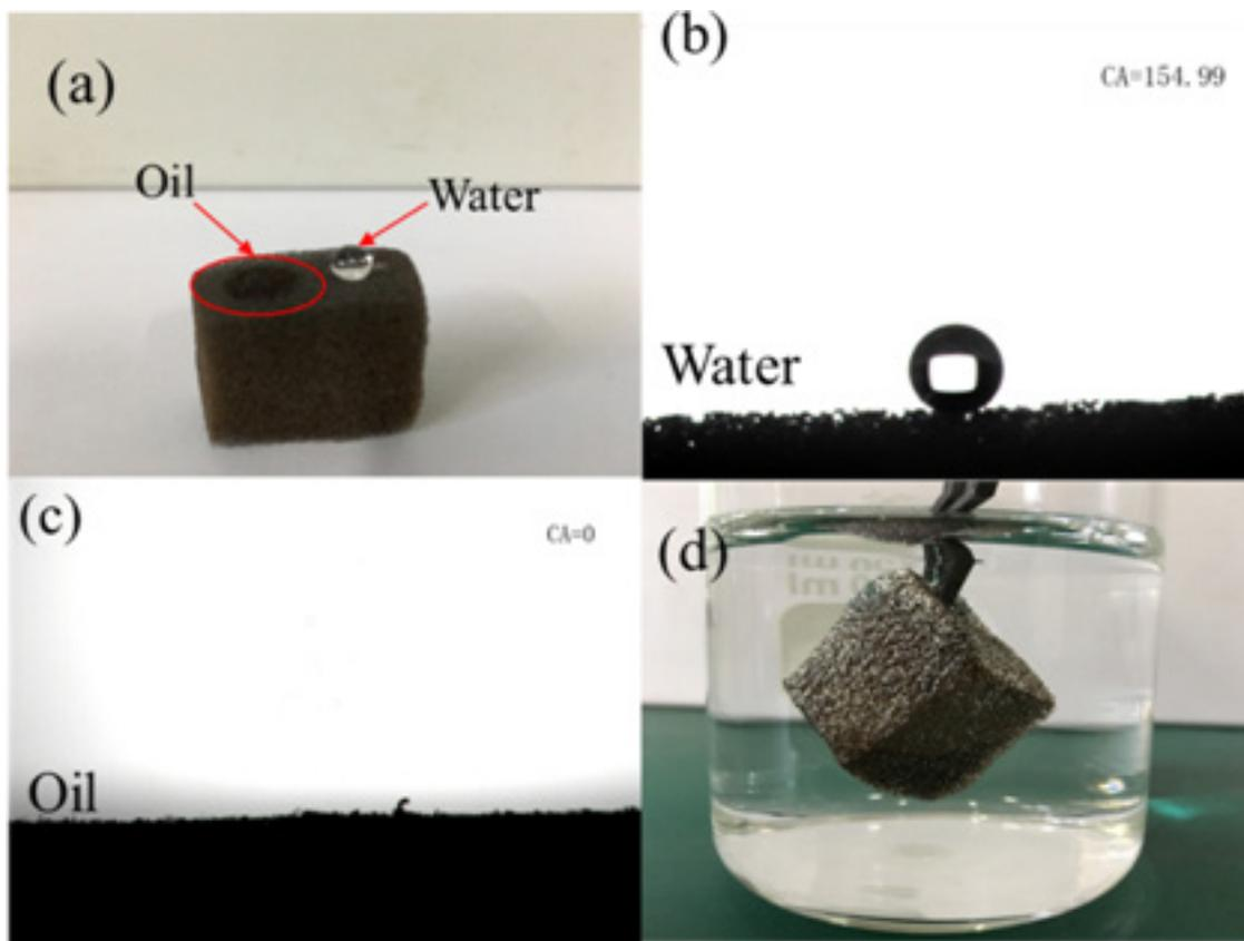
Fig. 4. (a) Water droplets and kerosene trace on the surface of the Ota-PDA-PU sponge. (b) Photograph of WAC on the surface of the FGP sponge. (c) Photograph of OAC on the surface of the FGP sponge. (d) Photograph of the Ota-PDA-PU sponge immersed in water by a force.
