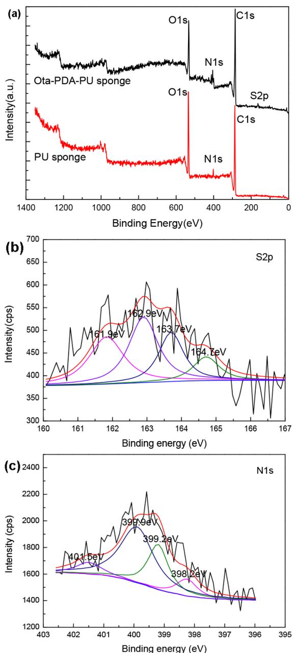
Fig. 2. (a) XPS survey scans of PU sponge and Ota-PDA-PU sponge, (b) S2p XPS spectrum of Ota-PDA-PU sponge and (c) N1s XPS spectrum of Ota-PDA-PU sponge.
