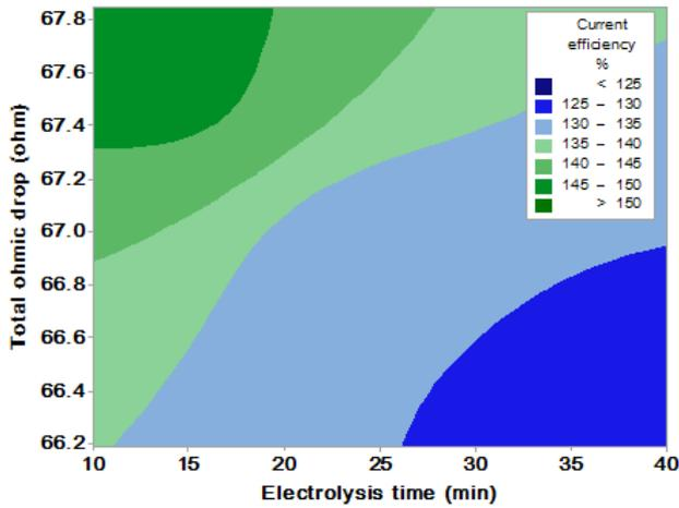
Fig. 6. Contour plot of current efficiency vs. total ohmic drop and electrolysis time.
