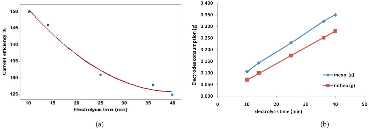
Fig. 4. (a) Current efficiency vs. electrolysis time (current density = 4.39 mA/cm<sup>2</sup>); (b) Experimental and theoretical electrodes consumption vs. electrolysis time (current density = 4.39 mA/cm<sup>2</sup>).
