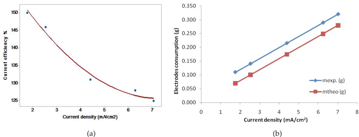
Fig. 8. (a) Current efficiency vs. current density (electrolysis time = 25 min); (b) Experimental and theoretical electrodes consumption vs. current density (electrolysis time = 25 min).
