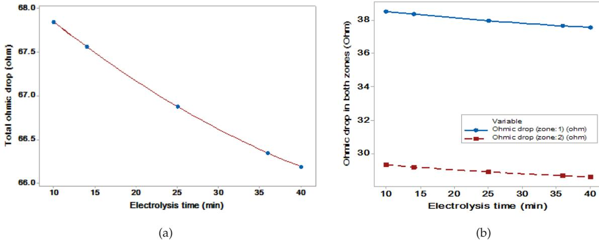
Fig. 5. (a) Total ohmic drop vs. electrolysis time (current density = 4.39 mA/cm<sup>2</sup>); (b) Ohmic drop in both zones vs. electrolysis time (current density = 4.39 mA/cm<sup>2</sup>).
