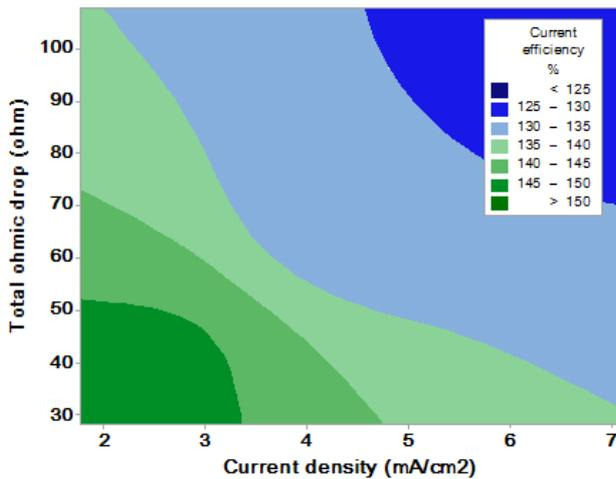
Fig. 10. Contour plot of current efficiency vs. total ohmic drop and current density.
