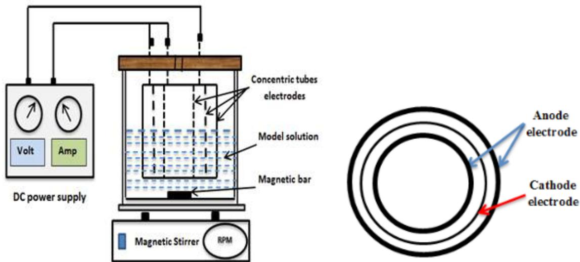
Fig. 3. Schematic of the electrocoagulation reactor and its electrodes.
