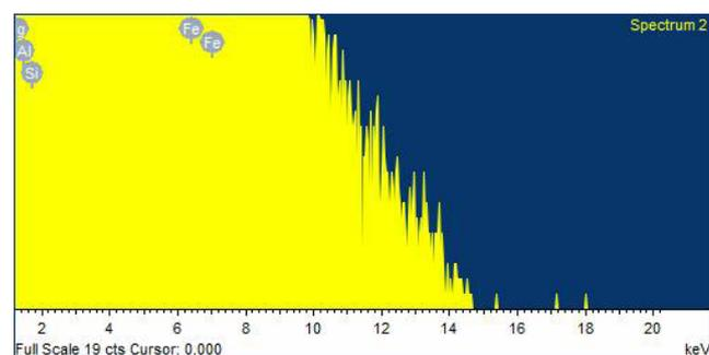
Fig. 2. Elemental composition of aluminum tube (EDS-test).
