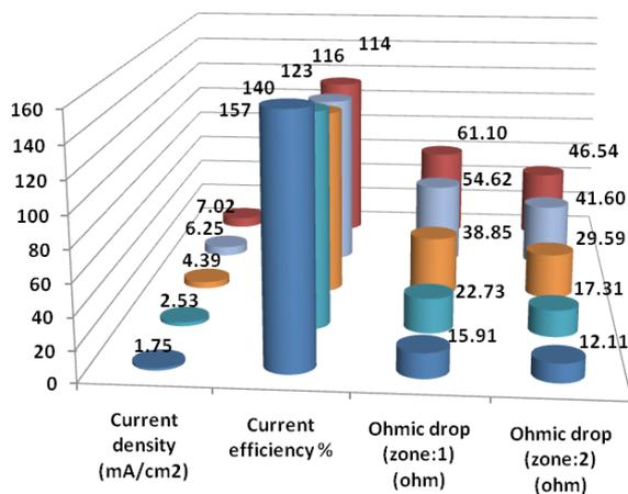
Fig. 11. Current efficiency vs. both zones of ohmic drop and current density.
