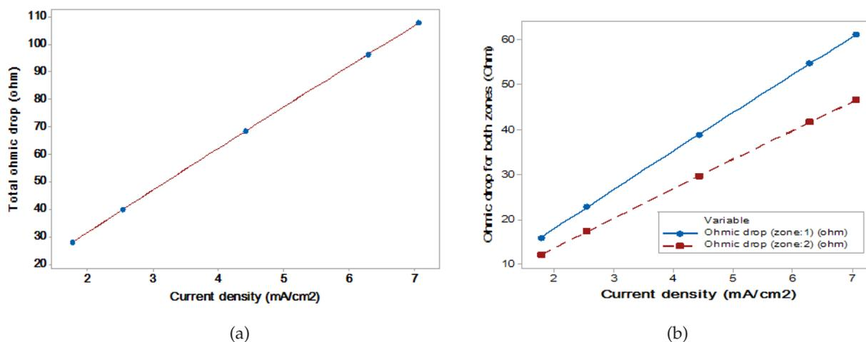
Fig. 9. (a) Total ohmic drop vs. current density (electrolysis time = 25 min); (b) Ohmic drop in both zones vs. current density (electrolysis time = 25 min).
