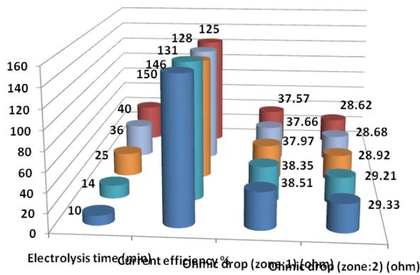
Fig. 7. Current efficiency vs. both zones of ohmic drop and electrolysis time.
