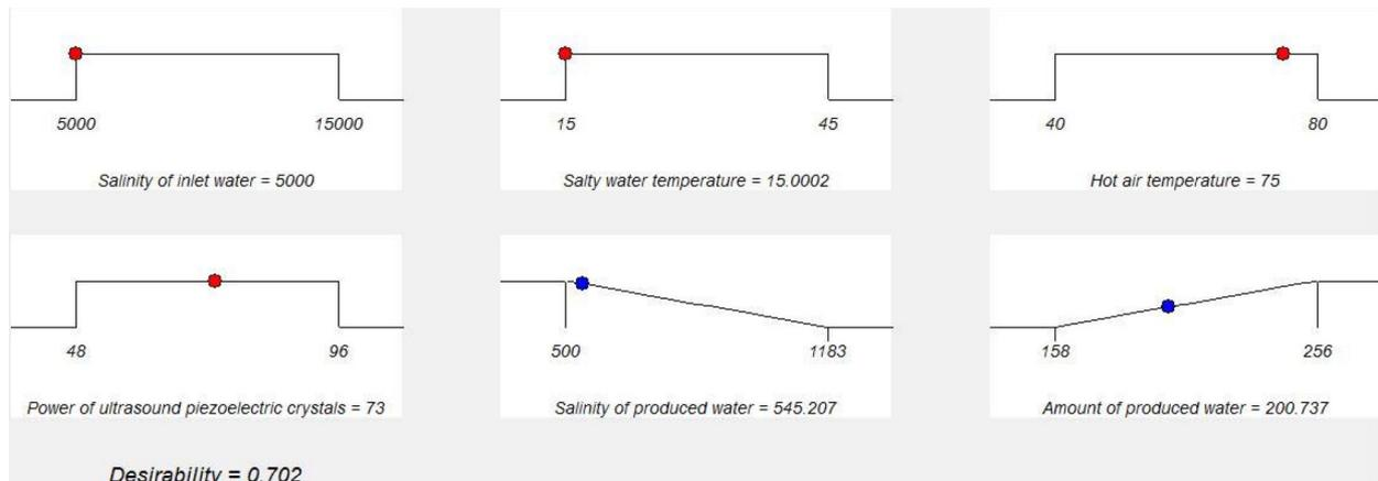
Fig. 5. The optimal levels of the operating parameters.
