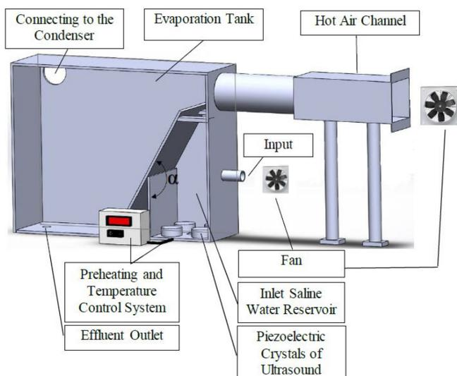
Fig. 1. Schematic view of ultrasonic desalination unit.
