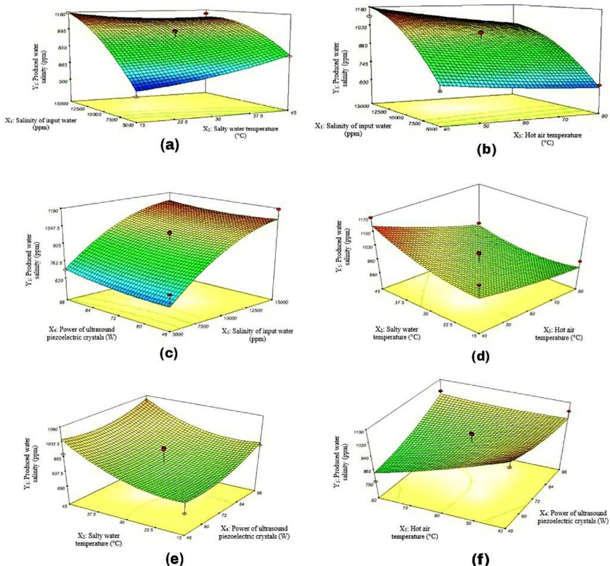
Fig. 3. Effect of interaction of operational parameters on produced water salinity.
