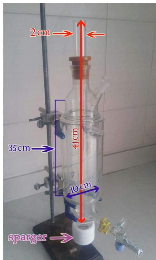
Fig. 1. The structure of the designed reactor.
