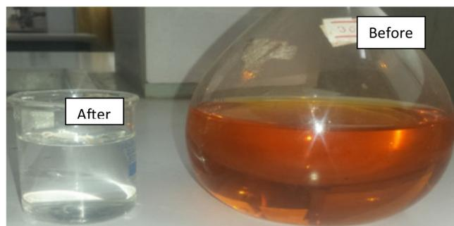
Fig. 6. Methyl-red aqueous solution before and after treatment with 25%  $H_2SO_4$  modified Zemer clay mineral.
