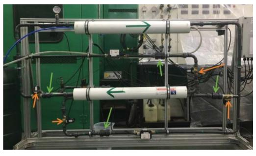
Fig. 3. Version 2 prototype: single-acting batch-RO system with electrically operated valves, at Aston University, UK. Yellow arrows indicate solenoid valves and green arrows indicate non-return valves.
