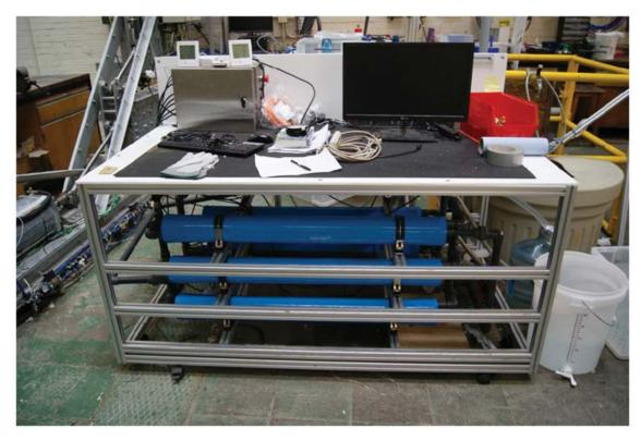
Fig. 5. Version 4 of the batch-RO prototype giving increased output through use of multiple vessels, at Aston University.
