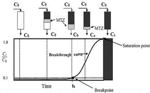
Fig. 1. Representation of a typical breakthrough curve.
