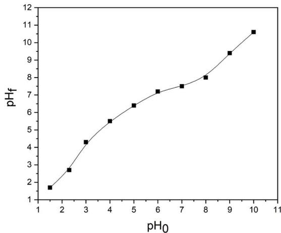
Fig. 4. Plot for determination of zero point charge for the RHS biosorbent.
