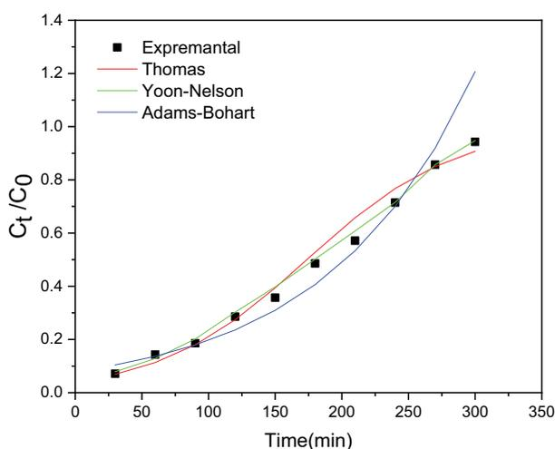
Fig. 11. Experimental and predicted breakthrough curves using the Thomas, Yoon–Nelson, and Adams–Bohart models for the sorption of Cr (VI) by RHA at an inlet hexavalent chromium concentration of 100 mg/L, flow rate 10 mL/min and bed height 4.3 cm.
