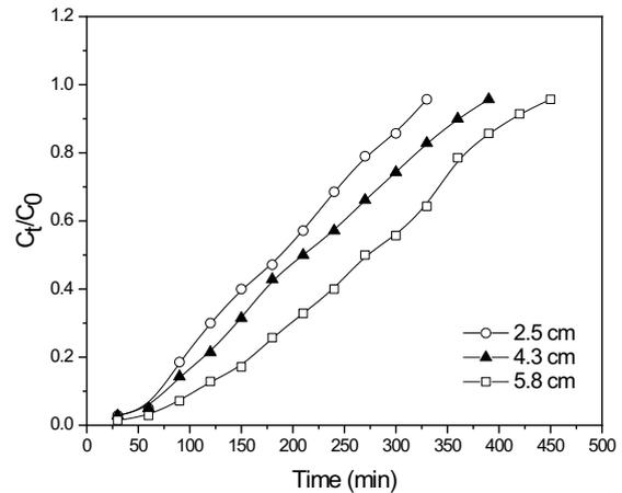
Fig. 5. Effect of various bed height on the breakthrough curve of Cr (VI) adsorption on RHA. Conditions: initial Cr (VI) concentration 100 mg/L; flow rate 5 mL/min; pH 2.5.
