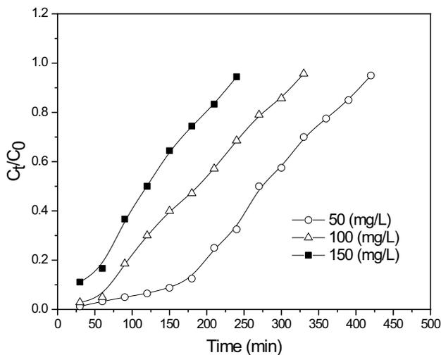
Fig. 7. Effect of initial Cr (VI) concentration on the breakthrough curve of Cr (VI) adsorption on RHA. Conditions: bed height 2.5 cm; flow rate 5 mL/min; pH 2.5.
