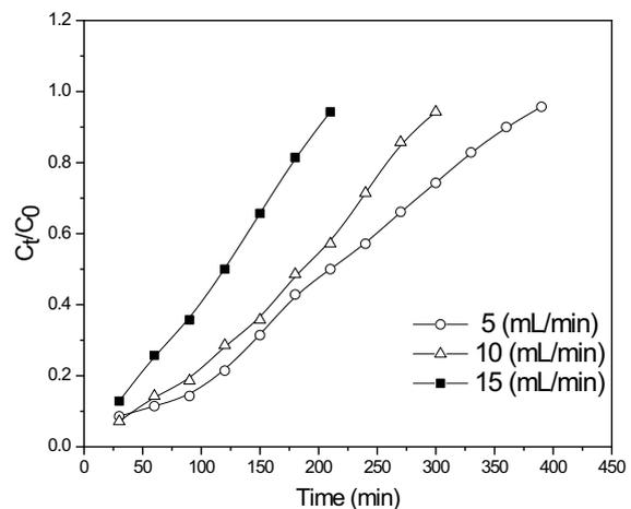
Fig. 6. Effect of various flow rates on the breakthrough curve of Cr (VI) adsorption on RHA. Conditions: bed height 4.3 cm; initial Cr (VI) concentration 100 mg/L; pH 2.5.
