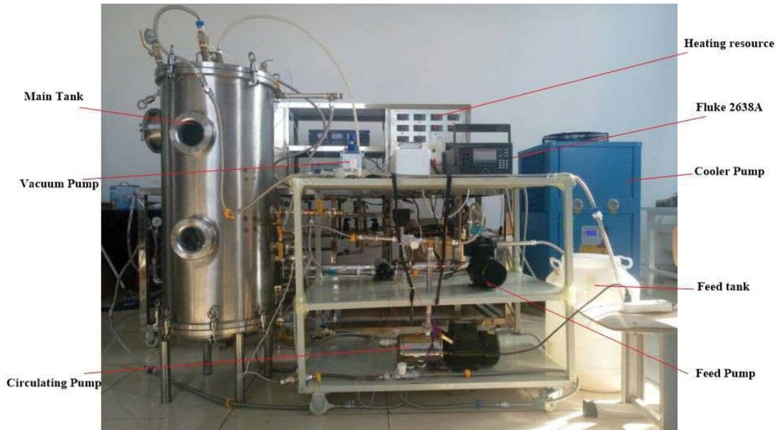
Fig. 2. Miniature low-temperature solar desalination setup.
