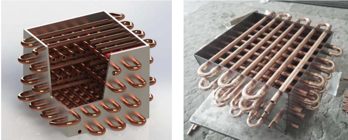
Fig. 4. Horizontal tube falling film evaporator.
