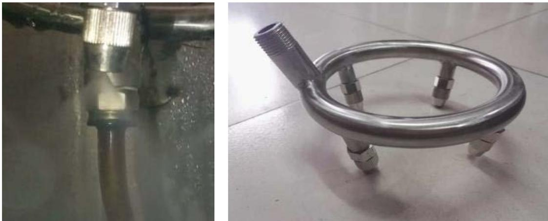
Fig. 6. Atomizing spray device.
