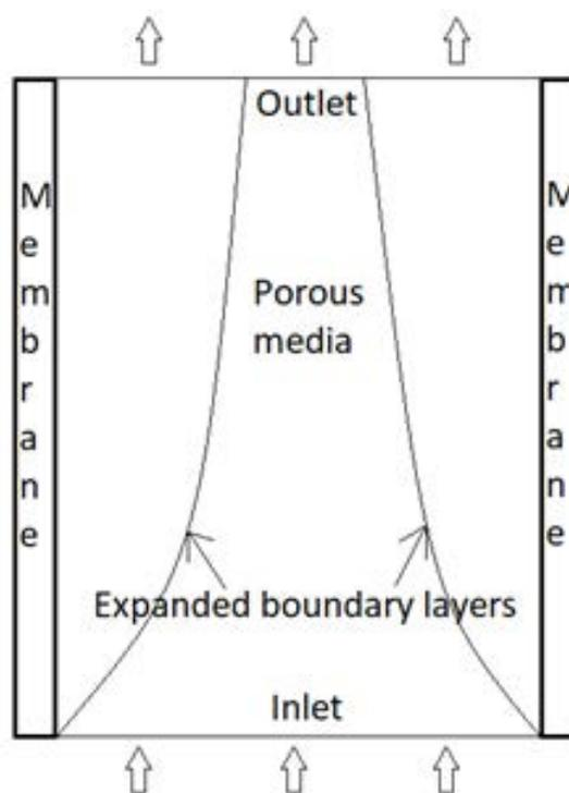
Fig. 1. Boundary layer expansion in porous media.
