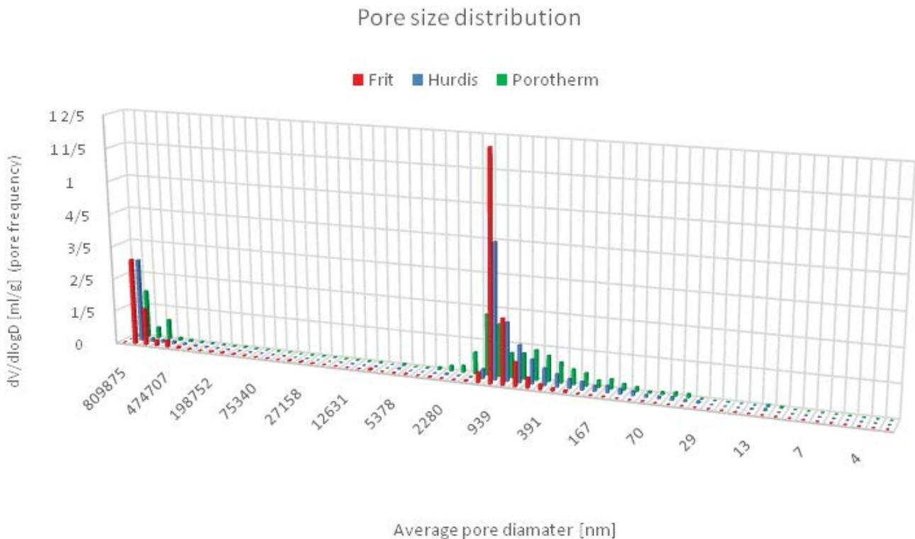
Fig. 3. Histogram of porous samples – Frit, Hurdis, Porotherm. Mercury porosimetry measured at The Unipetrol Centre for Research and Education (AutoPore IV 9510).
