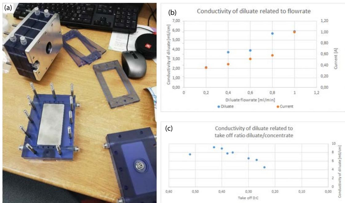
Fig. 9. (a) Shock electro dialysis unit "IV generation" (scalable – multiple chambers). and (b,c) conductivity of diluate related to flowrate and take off ratio diluate/concentrate. Inlet solution is Na<sub>2</sub>SO<sub>4</sub> with conductivity 14 mS cm<sup>-1</sup>. The IV generation 1-chamber unit (1 membrane pair – cat.ex).
