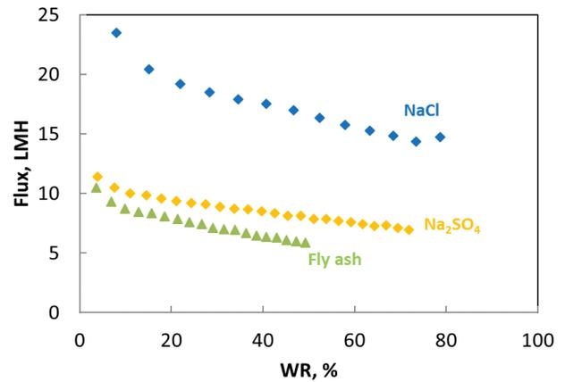
Fig. 3. Concentration of tannin using FO at 40°C. FO's draw solutions were 12 w-% NaCl, Na<sub>2</sub>SO<sub>4</sub> and fly ash from a soda recovery boiler.
