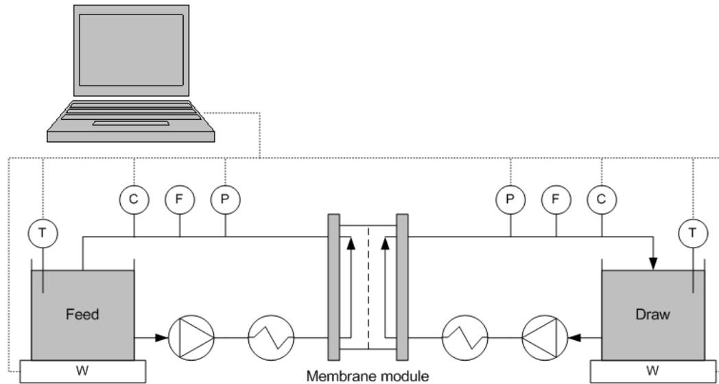
Fig. 1. Schematic figure of a laboratory scale FO testing apparatus with online data collection of weight ( $w$ ), temperature ( $T$ ) and conductivity ( $C$ ).
