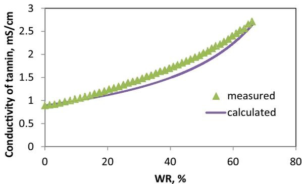
Fig. 5. Measured and calculated (from water recovery) conductivities of the feed solution during the FO process with a 20% soda ash draw solution at 40°C.
