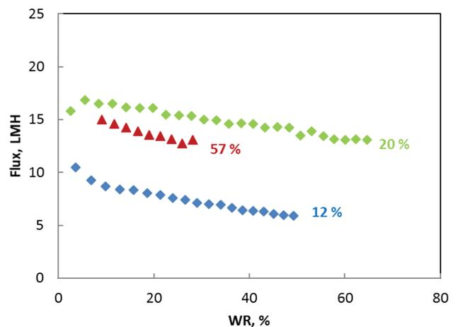
Fig. 4. Effect of the concentration of soda ash on the flux of FO, when the tannin solution acted as a feed solution.
