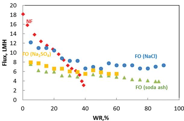
Fig. 2. Comparing membrane concentration methods for the tannin solution, that is, NF and FO, at 25°C. Draw solutions of FO were 12 w-% NaCl, Na<sub>2</sub>SO<sub>4</sub> and fly ash from the soda recovery boiler. When NF was used, operation pressure was 5 bar.
