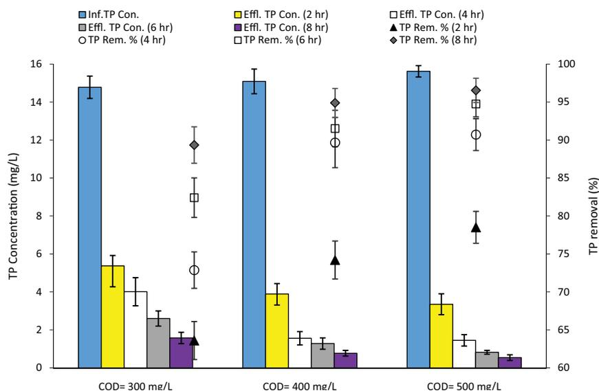
Fig. 4. Efficiency of modified Phoredox system in the relationship between phosphorus consumption and organic load (TP = 15 mg/L).
