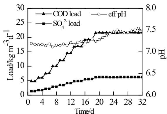
Fig. 2. Variation of effluent pH value with the load.
