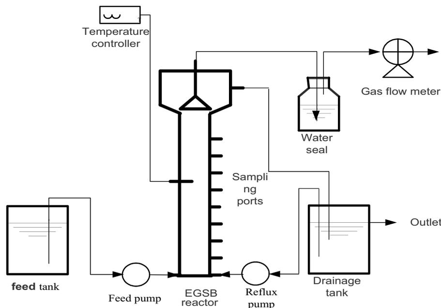
Fig. 1. Sketch of EGSB reactor system.
