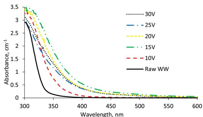
Fig. 5. Absorbance values of rinsing-wastewater and effluents of the dilute compartment in the ED process under different applied potentials.
