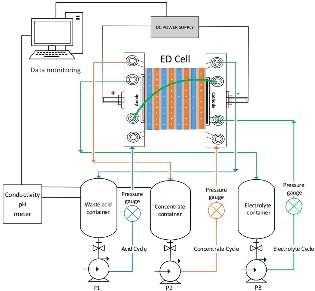
Fig. 1. Schematic representation of the batch electro dialysis process.
