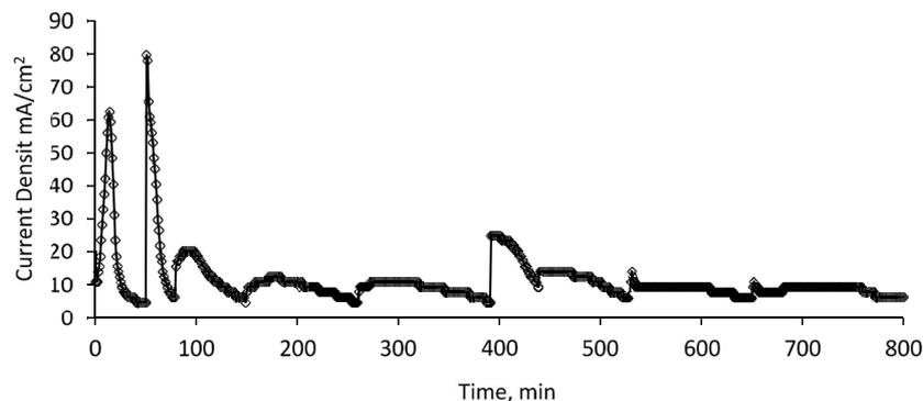
Fig. 7. Current density values for the continuous operation of the ED system without changing the concentrate compartment.
