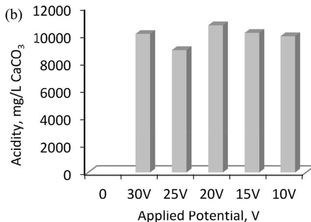
Fig. 4. Graphs of acidity vs. the applied potential for (a) the dilute compartment and (b) the concentrate compartment.
