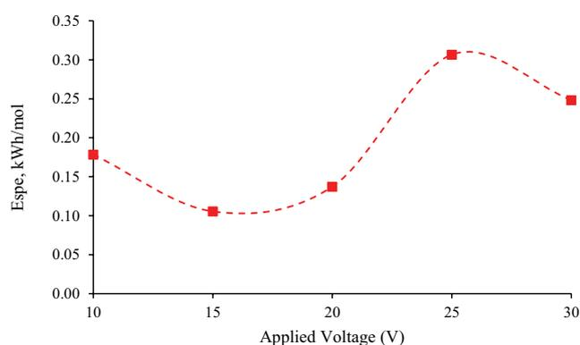
Fig. 9. Specific energy consumption of the ED process under applied potentials (10–30 V).
