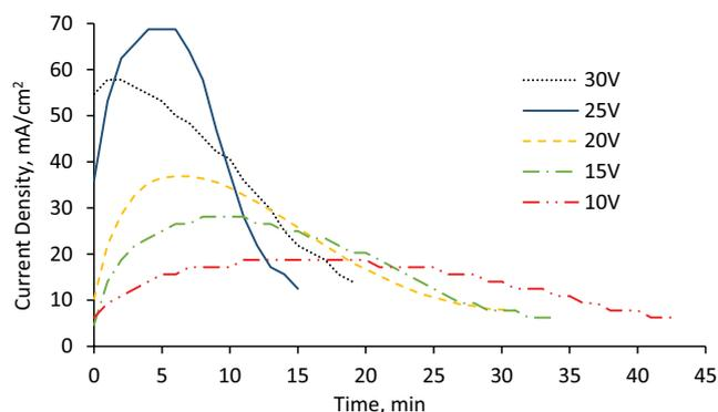
Fig. 8. Current density values for the continuous operation of the ED system without changing the concentrate compartment.
