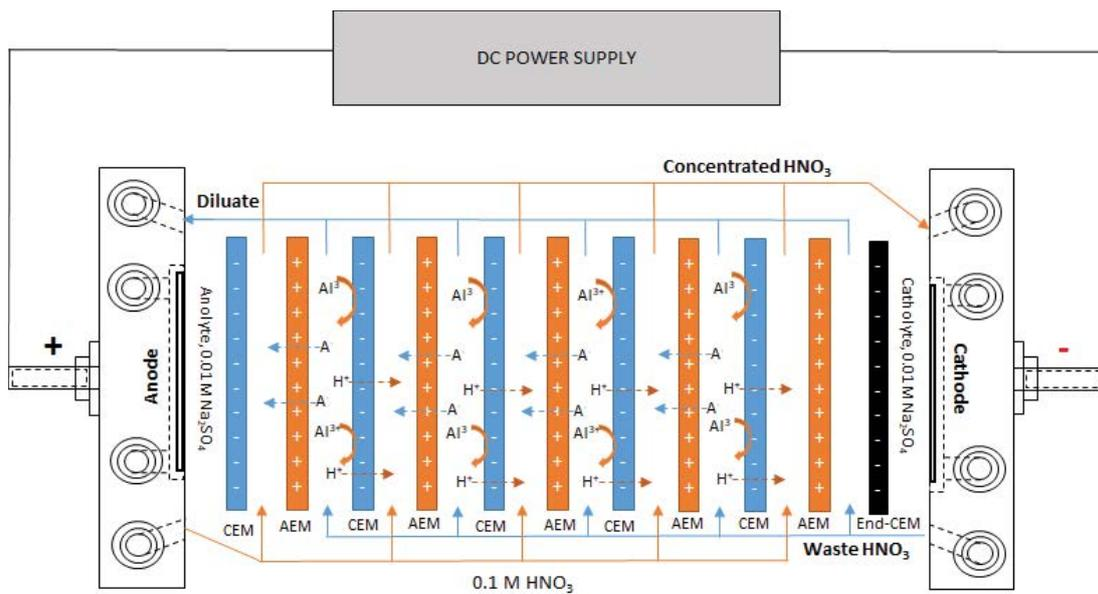
Fig. 2. Schematic representation of the ED cell configuration for recovery of waste acid. (CEM: cation exchange membrane, AEM: anion exchange membrane, End-CEM: end cation exchange membrane, A<sup>-</sup>: anion (NO<sub>3</sub><sup>-</sup> etc.).
