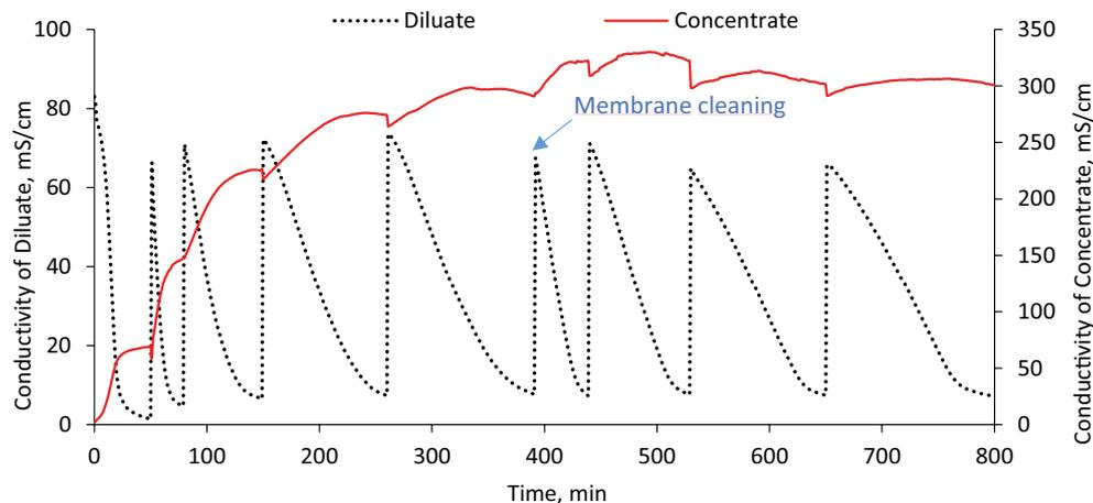
Fig. 6. Change in conductivity of concentrate and dilute compartments. The ED system was run with the same concentrate solution while the dilute solution was replaced when it reached to 8 mS/cm of conductivity value (The applied potential was 25 V).
