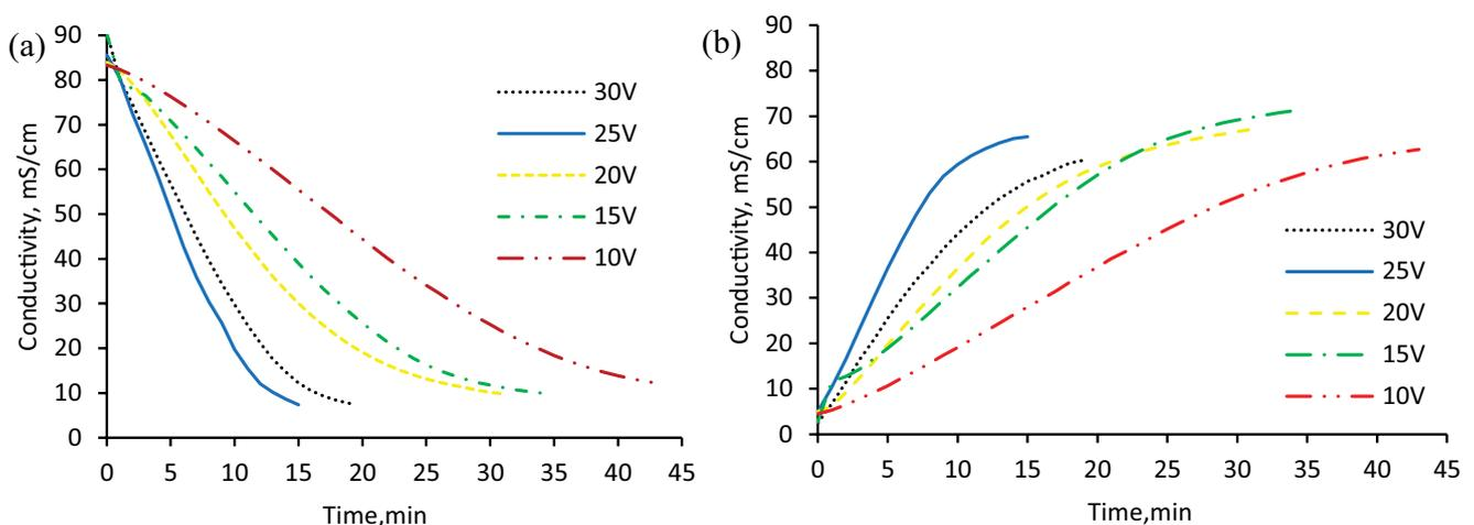
Fig. 3. Graphs of conductivity vs. time for the ED studies under various applied potential differences; (a) the dilute compartment and (b) the concentrate compartment.
