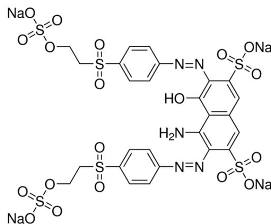
Fig. 1. Chemical structure of RB5 dye [7].
