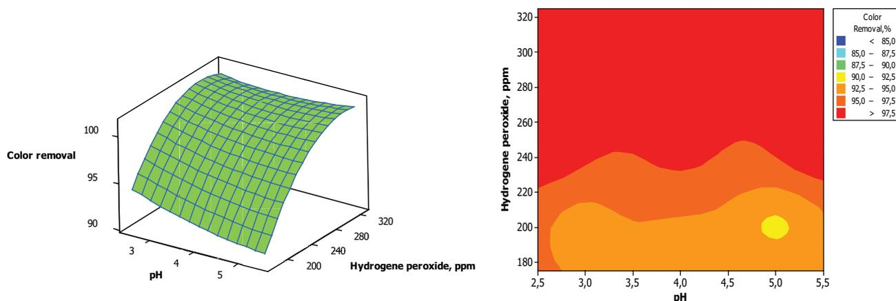
Fig. 7. Effect of initial solution pH to removal efficiency (constant dye concentration 200 ppm,  $\text{Fe}^{2+}$  40 ppm).
