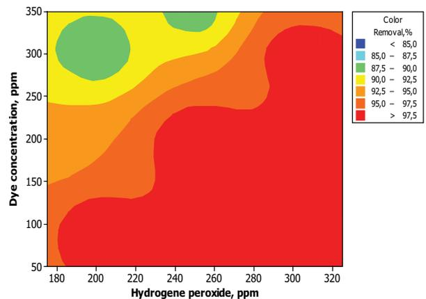
Fig. 6. Effect of hydrogen peroxide concentration on removal efficiency (constant pH 4, Fe<sup>2+</sup> 40 ppm).
