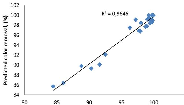
Fig. 2. Observed vs. predicted plot of color removal.
