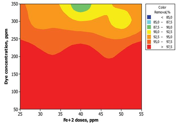
Fig. 5. Effect of iron ion concentration on removal efficiency (constant pH 4, H<sub>2</sub>O<sub>2</sub> 250 ppm).
