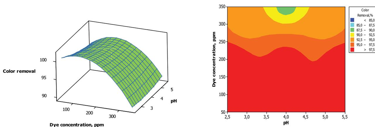
Fig. 8. Effect of RB5 dye concentration on removal efficiency (constant  $\text{H}_2\text{O}_2$  250 ppm,  $\text{Fe}^{2+}$  40 ppm).
