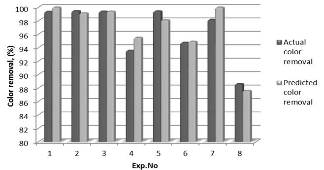
Fig. 3. Observed vs. predicted plot of color removal for eight new control experiments.
