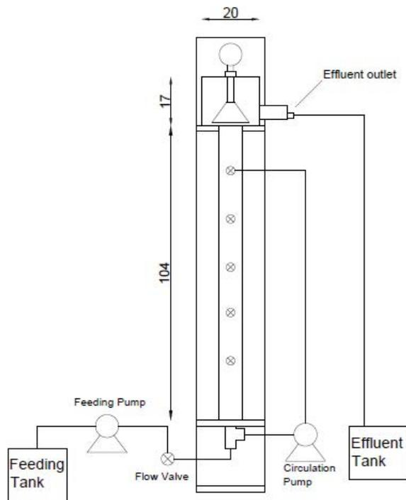
Fig. 1. EGSB reactor set up.
