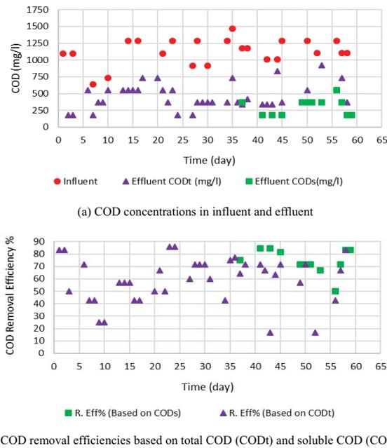
Fig. 2. COD removal from urine in the EGSB reactor (a) COD concentrations in influent and effluent and (b) COD removal efficiencies based on total COD (CODt) and soluble COD (CODs).
