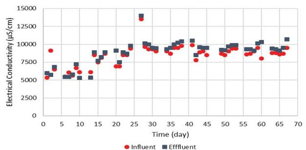
Fig. 6. Conductivity of influent and effluent of 25% fresh urine in μS/cm.
