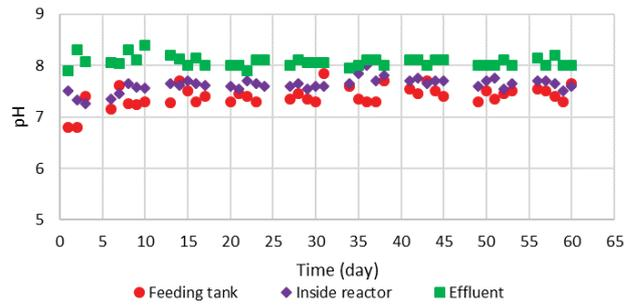
Fig. 3. pH values of the anaerobic system.
