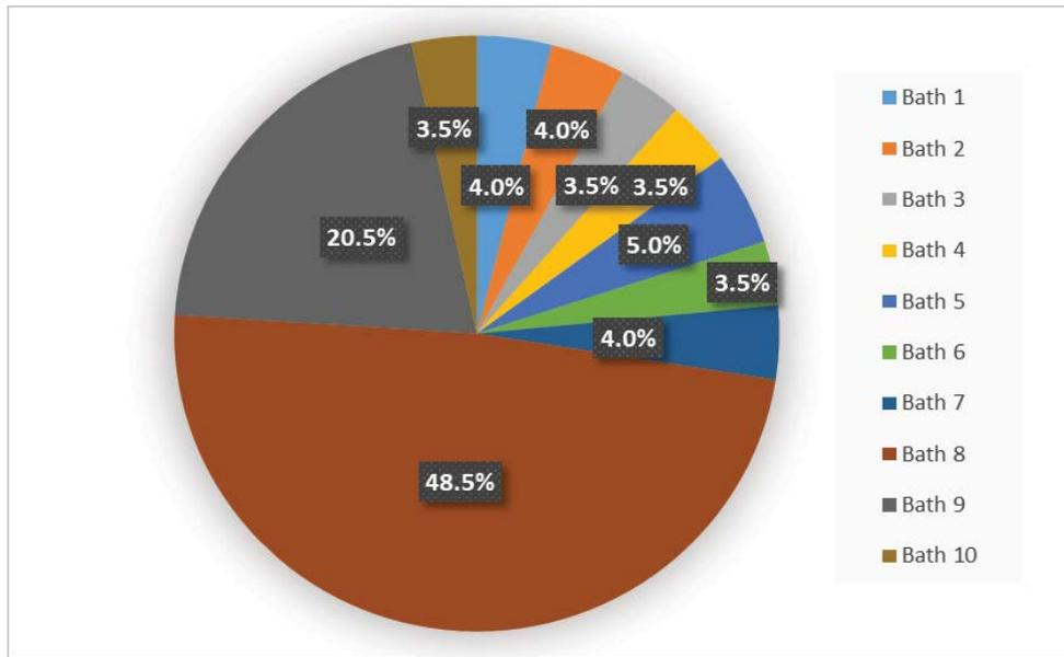
Fig. 2. Distribution of electricity consumption in cataphoresis process.
