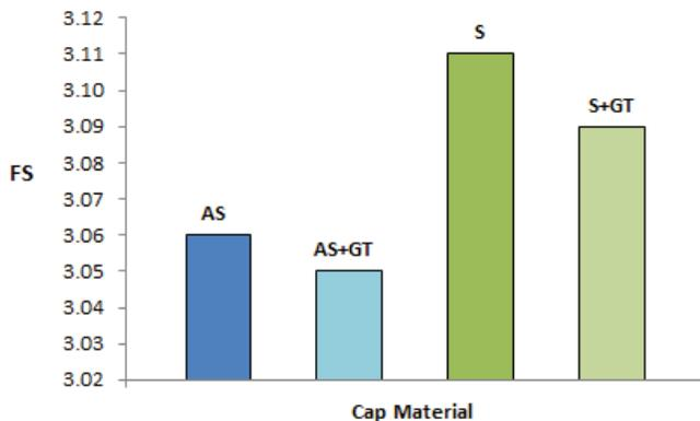
Fig. 6. FS values corresponding to different capping configurations.
