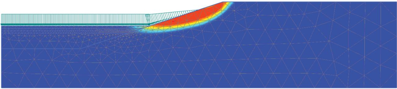
Fig. 5. Typical shadings of the total displacement increments indicating the most applicable failure mechanism of side slopes of the contaminated river bed.
