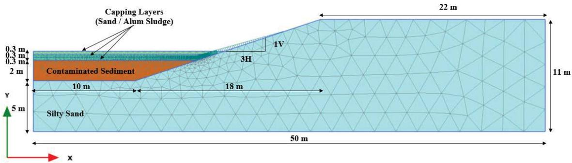
Fig. 2. Typical finite element mesh used to model the subaqueous contaminated sediment capping.
