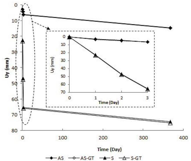
Fig. 3.  $U_y$  values of the contaminated sediment 365 d after the completion of the capping system.
