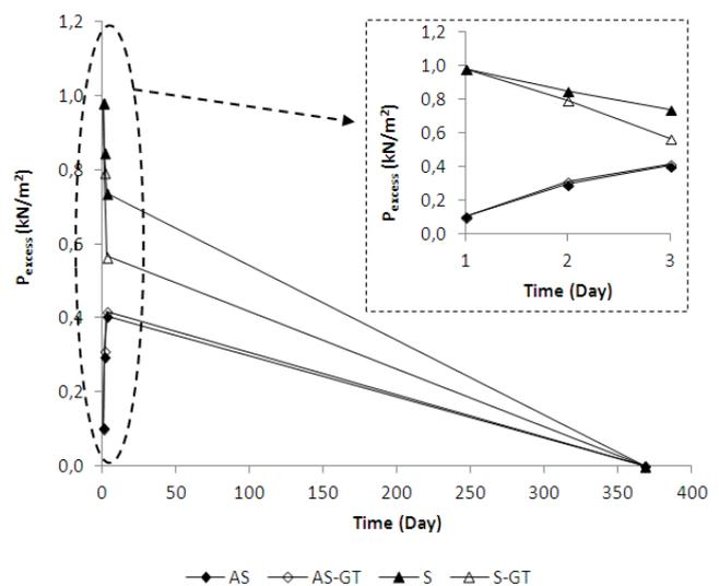
Fig. 4. Variation of the  $P_{\text{excess}}$  with time for different capping configurations.
