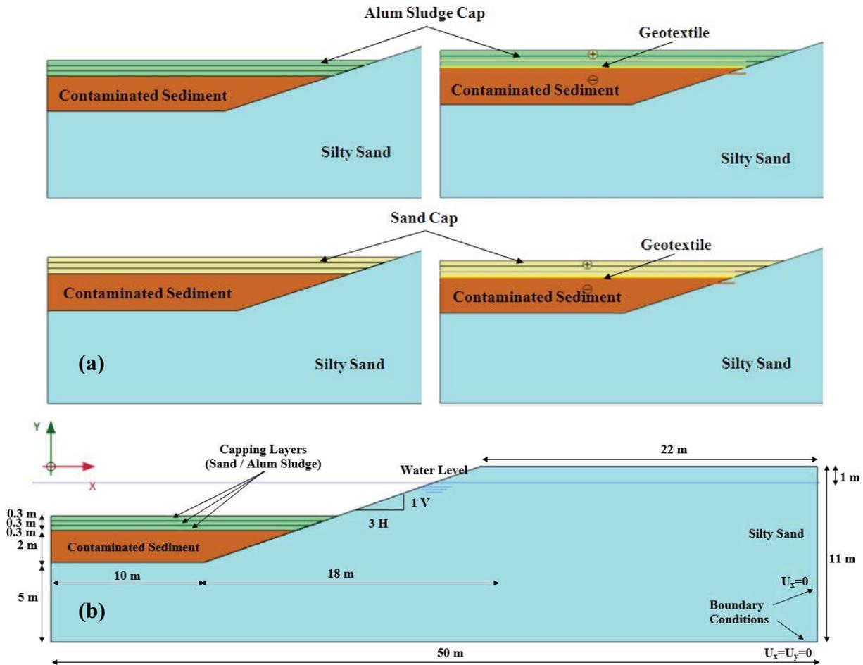
Fig. 1. (a) Details of the capping systems and (b) problem being analyzed.
