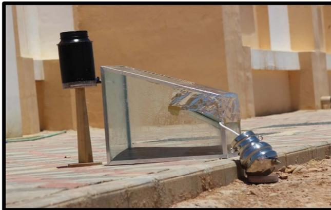
Fig. 2. Picture of the manufactured solar distiller.
