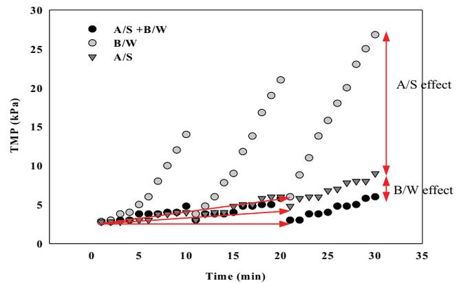
Fig. 2. Fouling properties with/without A/S and B/W.
