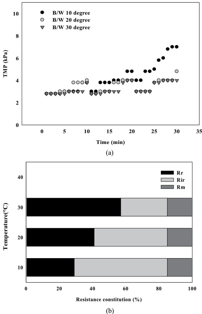
Fig. 6. (a) Compare of operating TMP and (b) membrane fouling resistance at different backwashing temperatures.
