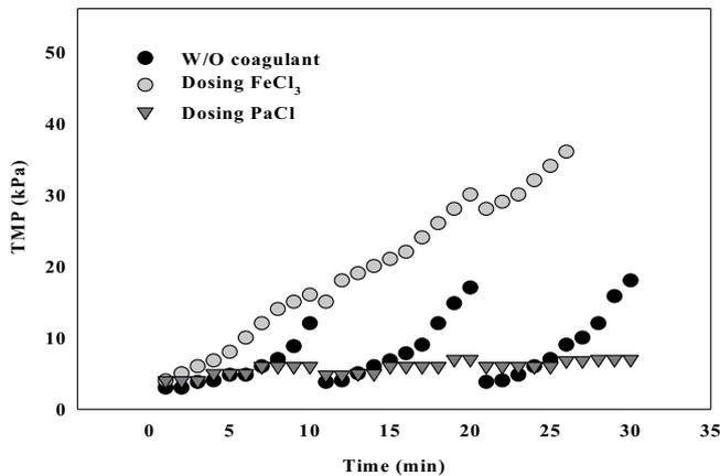
Fig. 1. Comparison of operating TMP by coagulant type and with/without injection of coagulants.
