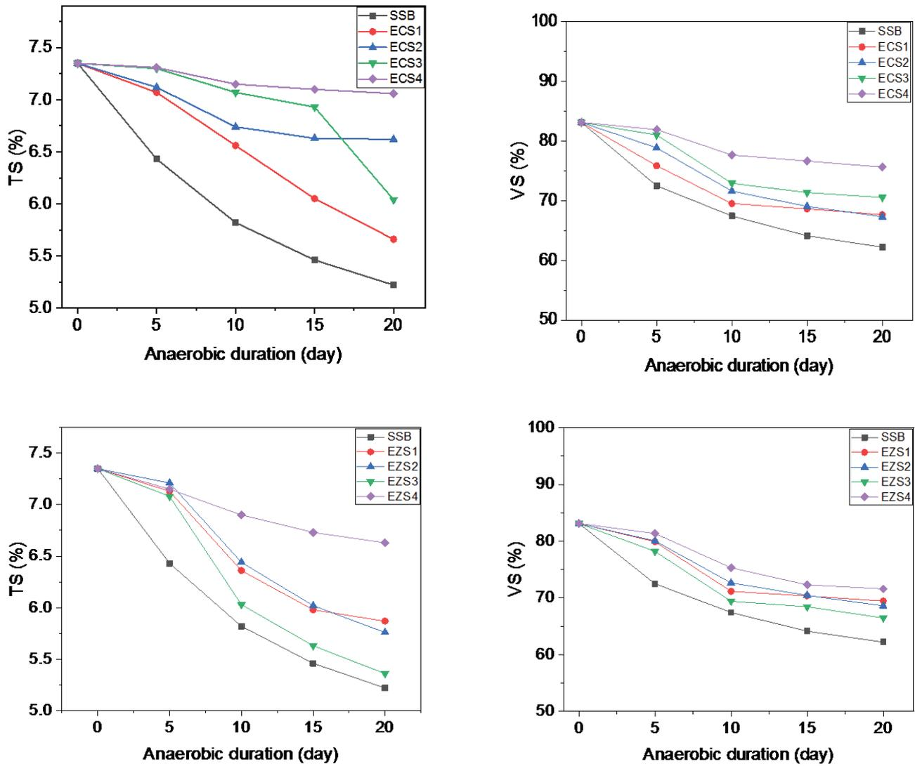
Fig. 2. Effects of copper and zinc on total solids and volatile solid removal.
