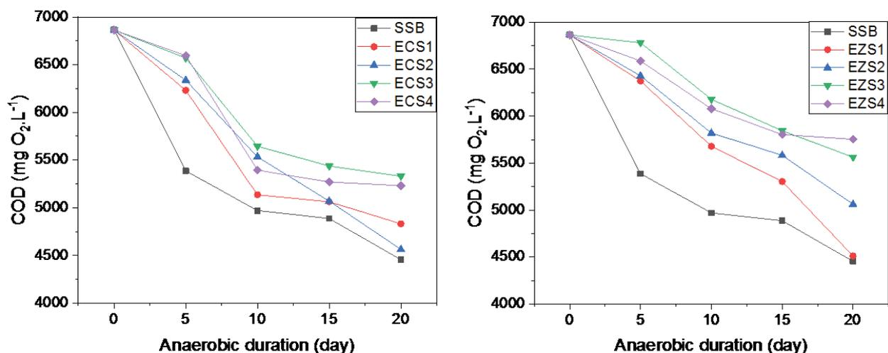
Fig. 3. COD removal during anaerobic digestion without and with the presence of copper and zinc.
