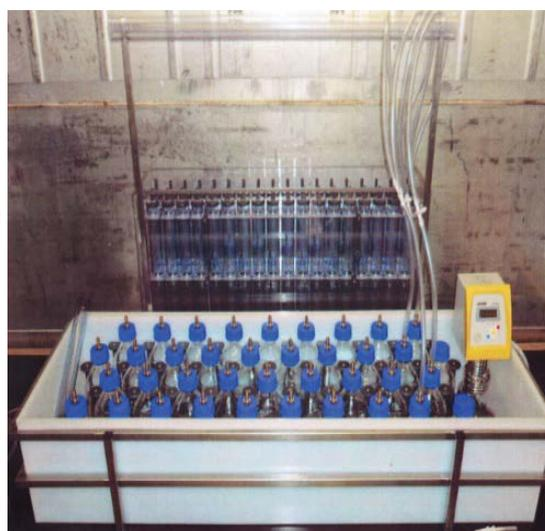
Fig. 1. Anaerobic batch tests digestion.
