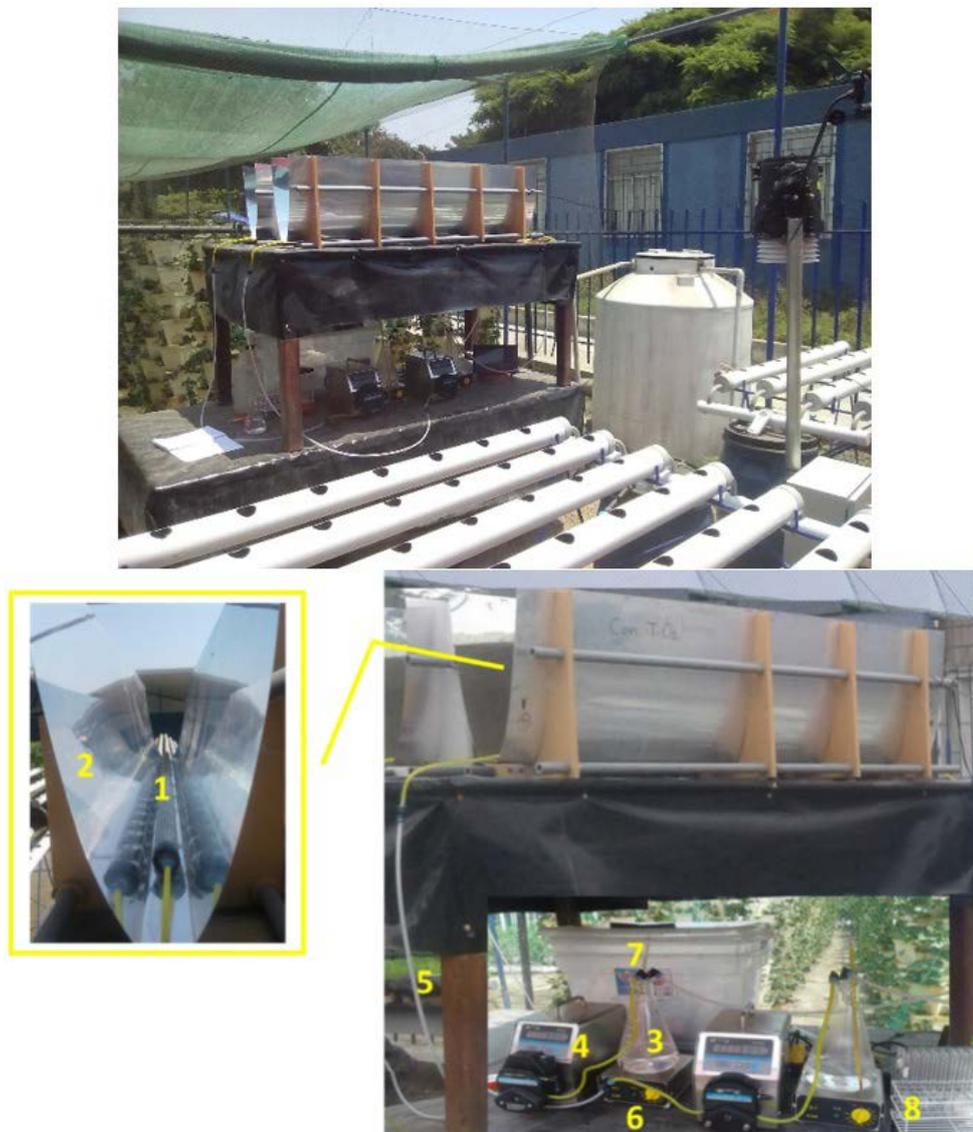
Fig. 4. Left: Photograph of the solar photocatalytic reactor. Center: 1, TCPC; 2, disinfection chamber containing the static mixer. Right: 3, 1 L Erlenmeyer flask; 4, peristaltic pump; 5, connection hoses; 6, magnetic stirrer; 7, mercury thermometer (0°C–150°C); 8, 16 × 100 mm test tubes used for sample collection.
