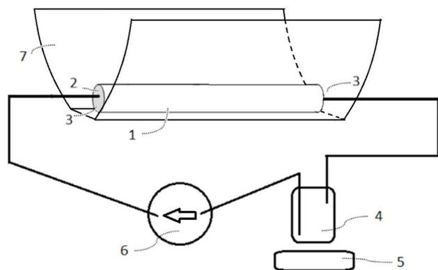
Fig. 1. Solar photocatalytic reactor. 1, Disinfection chamber; 2, Air-tight sealing lid; 3, Water inlet and outlet ports; 4, Container with a temperature sensor; 5, Magnetic stirrer; 6, Peristaltic pump; 7, Truncated compound parabolic concentrator.
