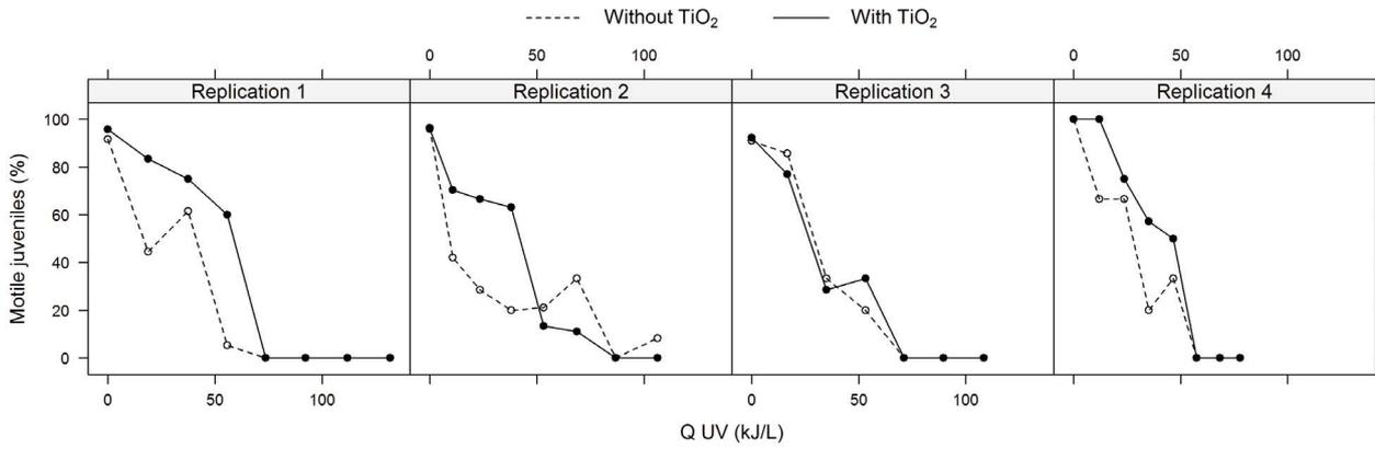
Fig. 7. Percentage of *Meloidogyne incognita* motile juveniles as a function of the  $Q_{UV}$  under solar radiation in a photoreactor with and without TiO<sub>2</sub>.
