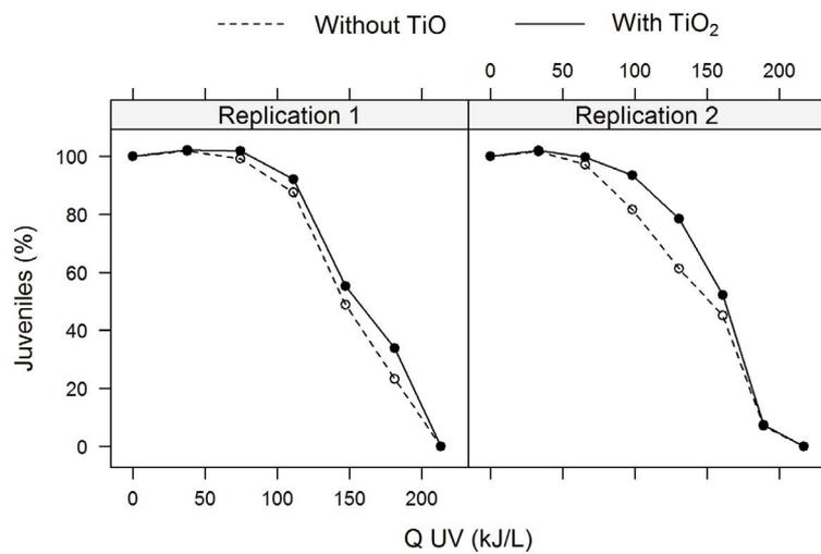
Fig. 8. Percentage of *Meloidogyne incognita* motile juveniles after egg hatching as a function of the  $Q_{UV}$  under solar radiation in a photoreactor with and without TiO<sub>2</sub>.
