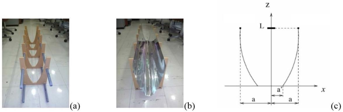
Fig. 3. (a) Photographs of the structure (with 3D-printed profiles and PVC pipes), (b) TCPC used in the solar photoreactor, and (c) dimensions of TCPC
