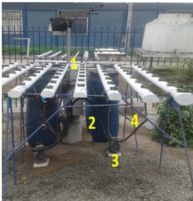
Fig. 5. Nutrient film technique hydroponic system; 1, pots with lettuce seedlings; 2, nutrient solution storage tank; 3,  $\frac{1}{2}$  HP pump; 4, recirculation hoses.
