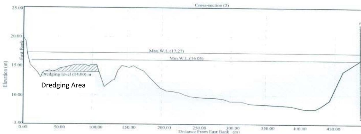
Fig. 11. Cross-section 5 at third intake Rod El Farag, [12].
