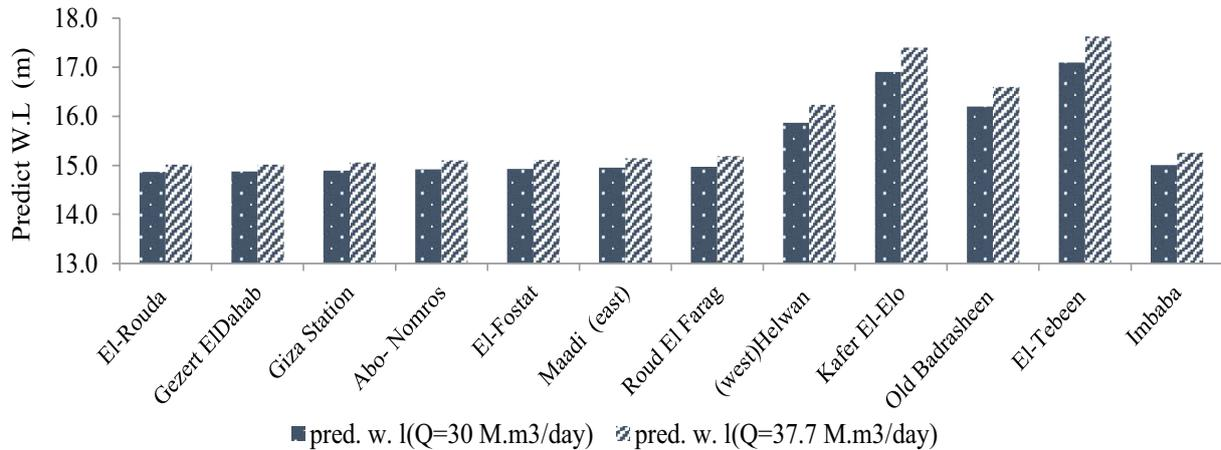
Fig. 7. The output of the hydraulic model at some of the drinking water stations.
