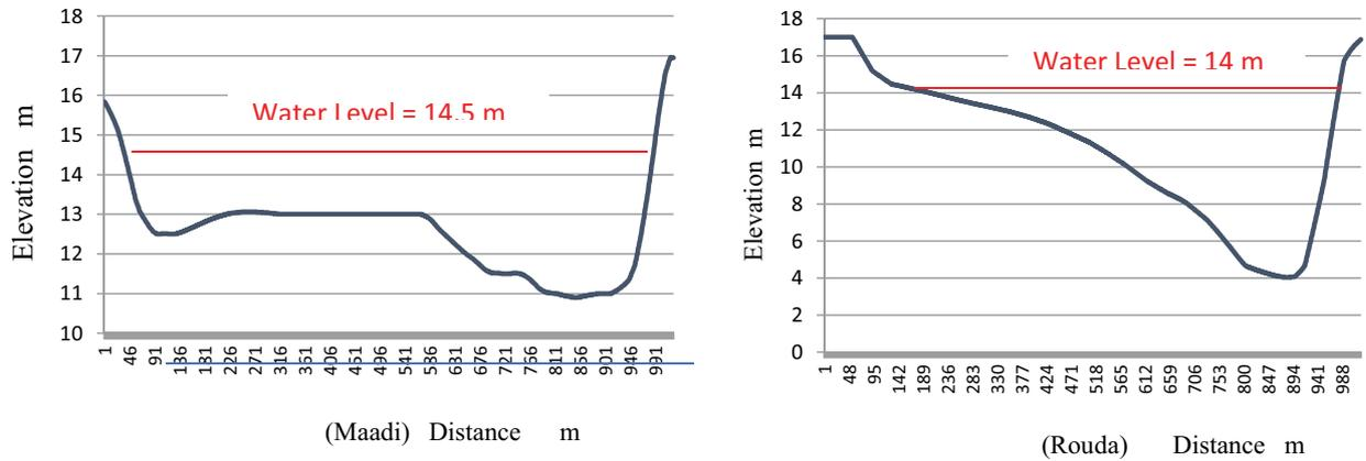
Fig. 10. Cross-sections at El Maadi and Rouda intakes.
