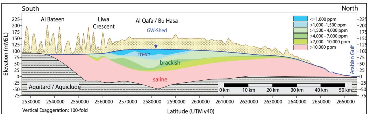
Fig. 5. Hydrogeological cross-section for the selected area.
