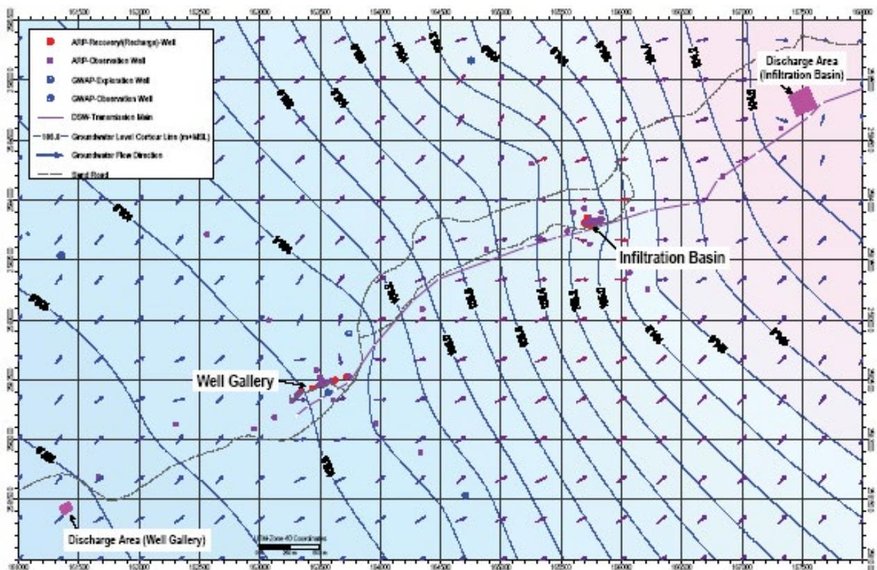
Fig. 6. Groundwater levels contour map (before injection, 2001).
