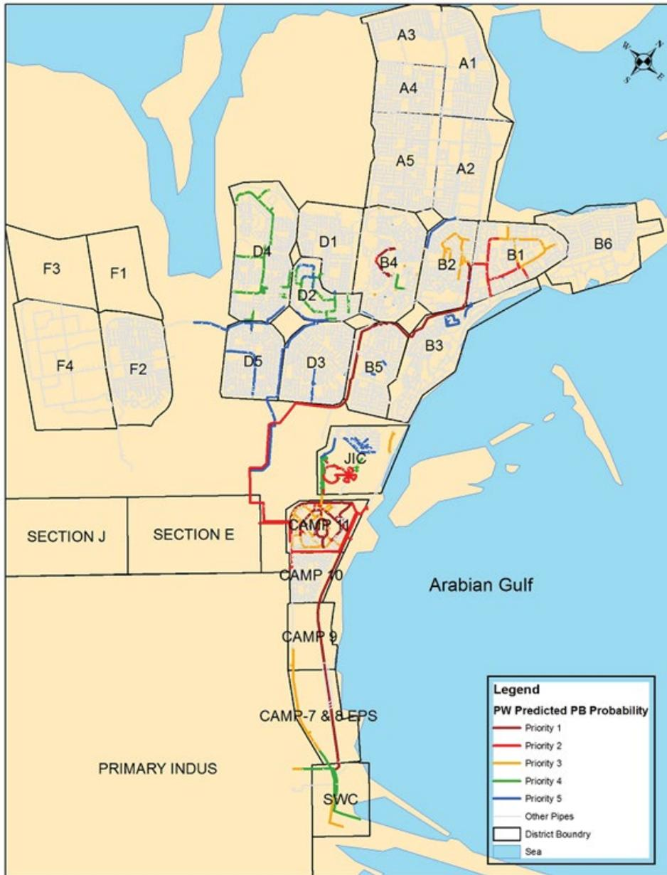
Fig. 4. Map of the potable water critical pipes based on high predicted pipe break probability,  $Pred(Pipe\_Breaks = 1) = \exp(z) / [1 + \exp(z)]$ .
