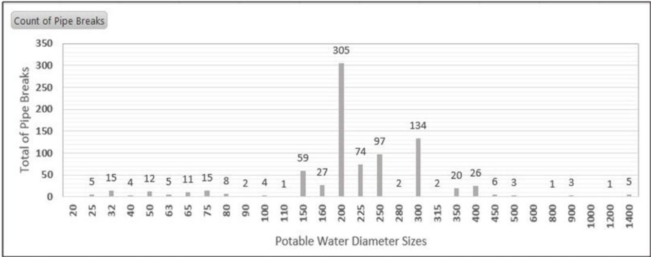
Fig. 2. Total potable water network pipe breaks according to the diameter sizes of the pipes.
