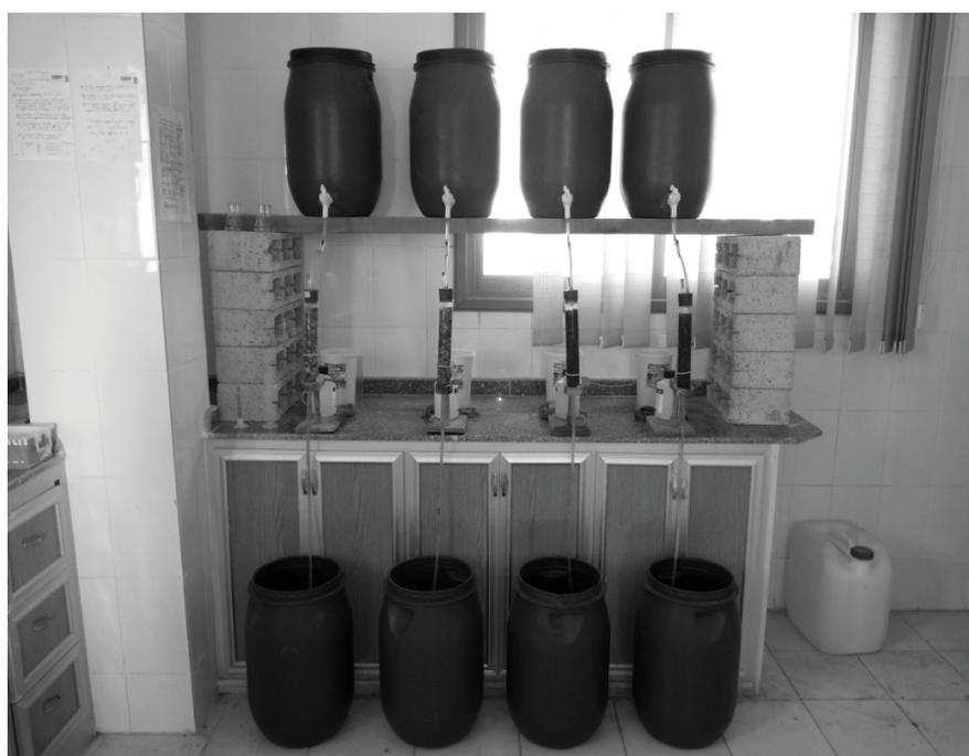
Fig. 2. Design of the percolating PVC and gravel microcosm.
