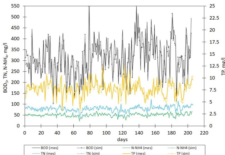
Fig. 2. Comparison of calculation results with measurements of selected wastewater quality indicators ( $BOD_5$ , TN,  $N-NH_4$ , TP) for the Sitkówka–Nowiny WWTP in the period covered by the measurements.
