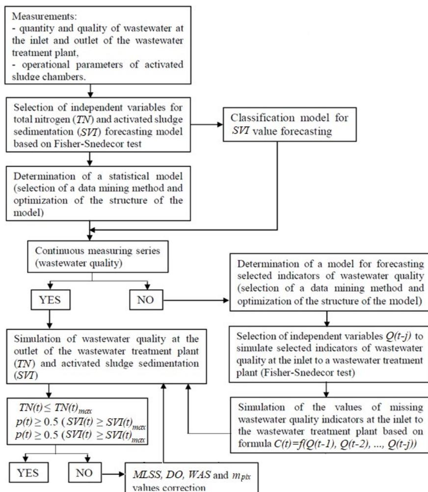
Fig. 1. Calculation scheme to determine a model for simulation, optimization, and control of WWTP operation (nitrogen removal, sedimentation of sludge in the secondary clarifier) in case of discontinuity of selected wastewater quality indicators.
