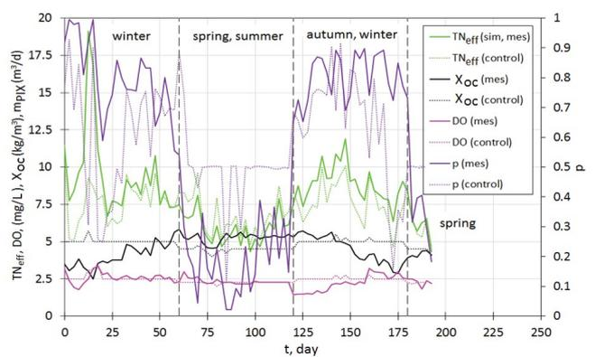
Fig. 6. Results of  $TN_{eff}$  and  $p$  calculations for the existing state of the process and after its optimization and the setting values in the bioreactor assuming discontinuity of the collected data.
