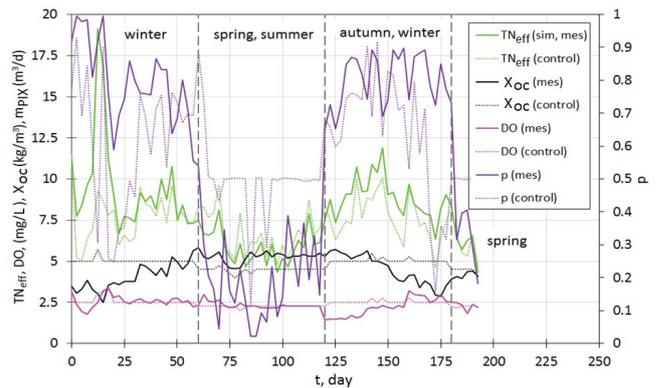
Fig. 5. Results of  $TN_{eff}$  and  $p$  calculations for the current state of the process and after its optimization and for the settings in the bioreactor with the assumption of continuity of the collected data.
