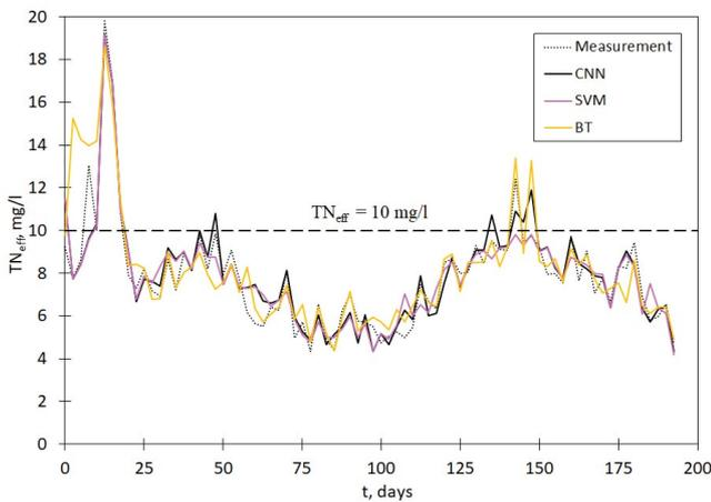
Fig. 3. Comparison of TN value measurements and calculation results obtained with CNN, SVM and BT models during the measurement period.
