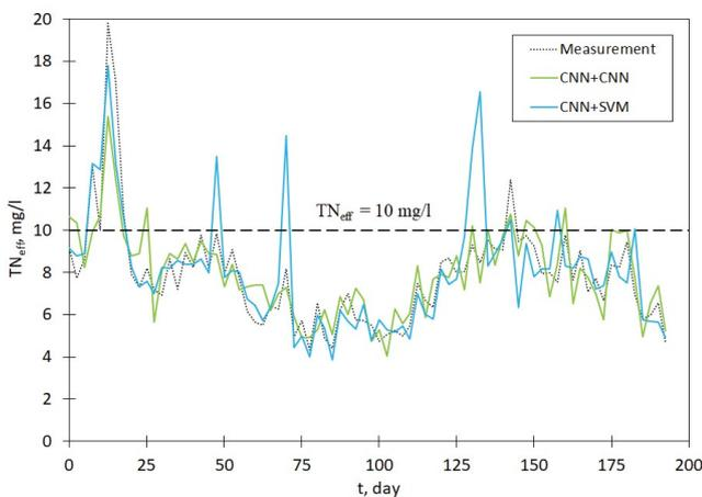
Fig. 4. Comparison of the TN value measurements and calculation results obtained with the CNN + CNN and CNN + SVM models during the measurement period.
