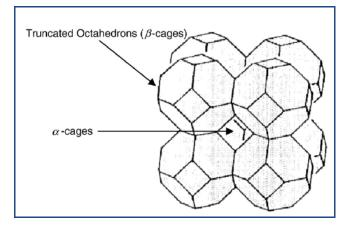
Fig. 2. Repeating unit of zeolite HS. Source, [23].
