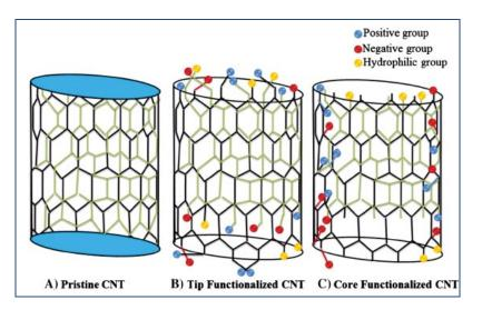
Fig. 6. Functionalization of CNT membranes. (a) Pristine CT, (b) tip functionalized CNT, and (c) core functionalized CNT. Source, [28].
