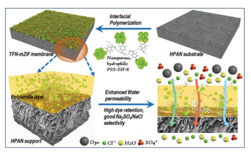
Fig. 1. Schematic of a TFN membrane containing poly (sodium 4 styrenesulfonate; PSS) modified ZIF-8 (mZIF) in a polyamide (PA) layer were constructed. Source, [17].
