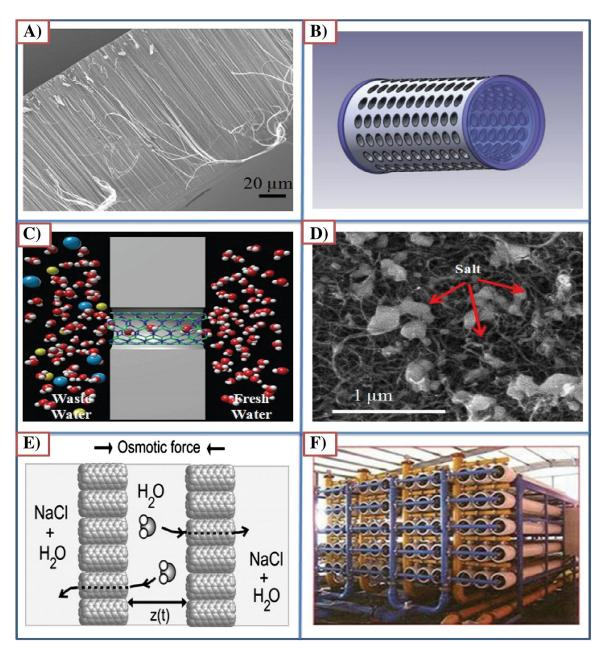
Fig. 5. Structures of some CNT membranes. Shown are (a) cross-sectional scanning electron microscope (SEM) image of a pristine CNT membrane; (b) CNT based water filter with cylindrical geometry; (c) movement of water molecules through a CNT channel; (d) SEM image of scattered NaCl nanocrystals on CNT membrane surface; (e) movement of pure water molecules through CNT-membrane in osmotically imbalanced compartments, and (f) engineered CNT membranes in industrial set up. Source, [28].
