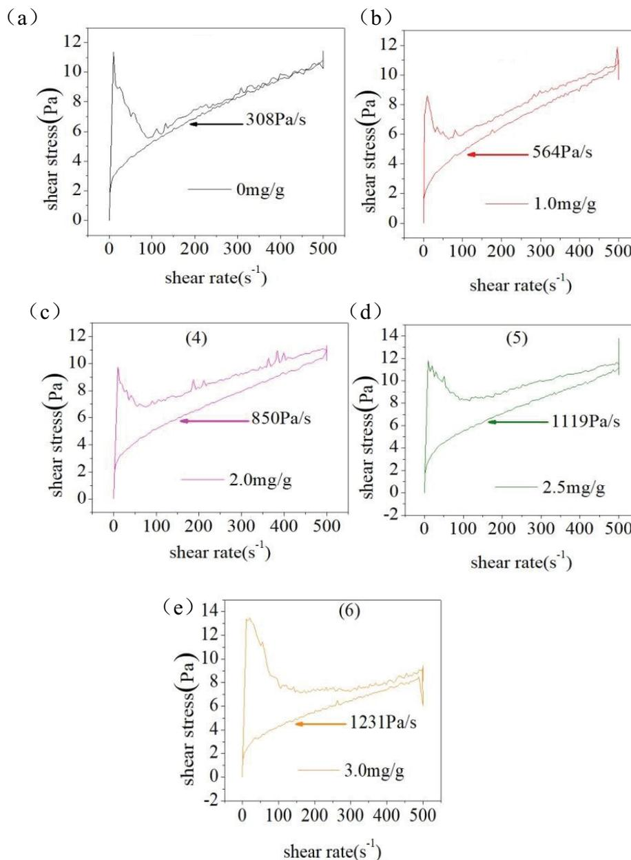
Fig. 4. Impact of CPAM dosage on thixotropy.
