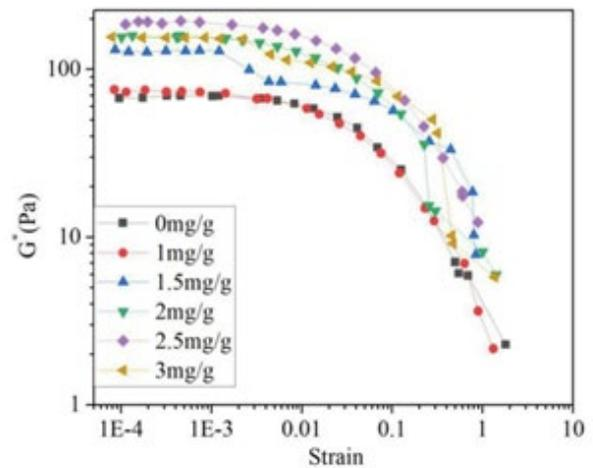
Fig. 5. Impact of CPAM on composite modulus.
