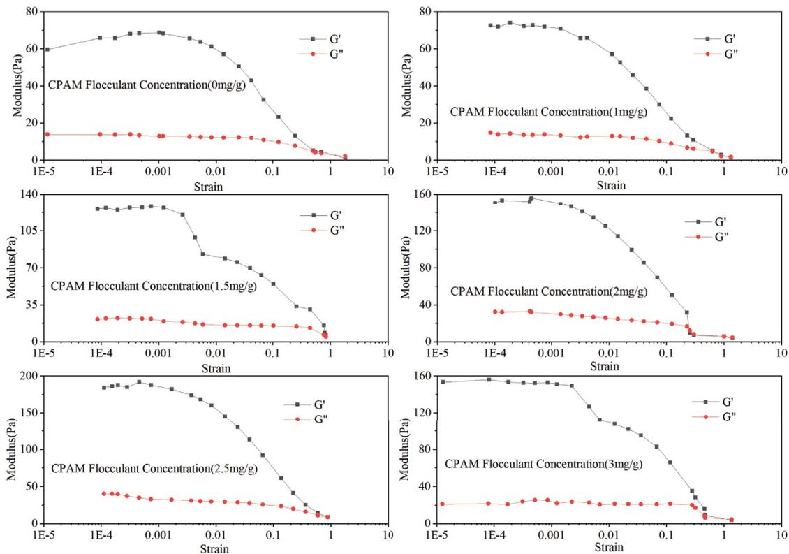
Fig. 6. Impact of CPAM on elastic and viscous modulus.
