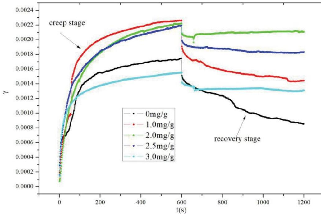
Fig. 7. Impact of CPAM flocculant dosage on creep recovery tests.
