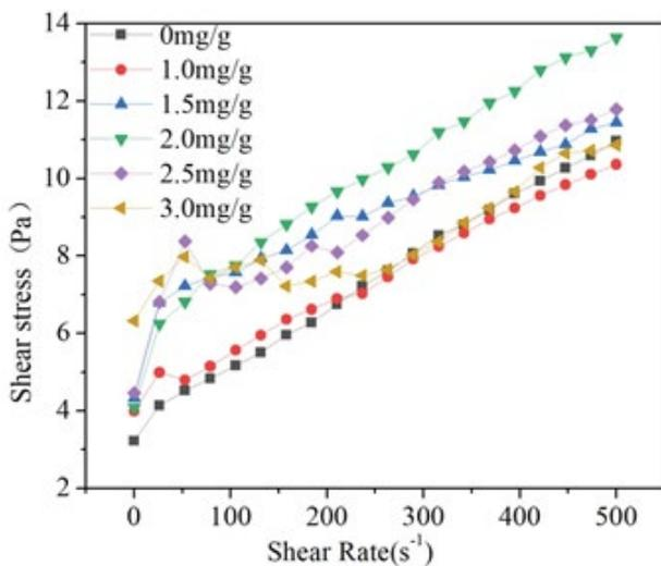
Fig. 2. Impact of flocculant CPAM dosage on a steady shear test.
