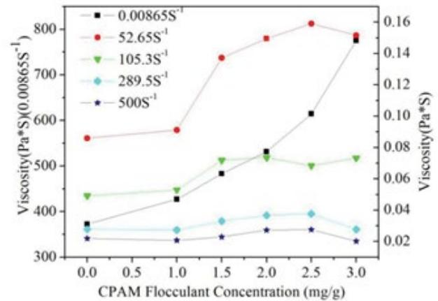
Fig. 3. Impact of flocculant CPAM dosage on viscosity.
