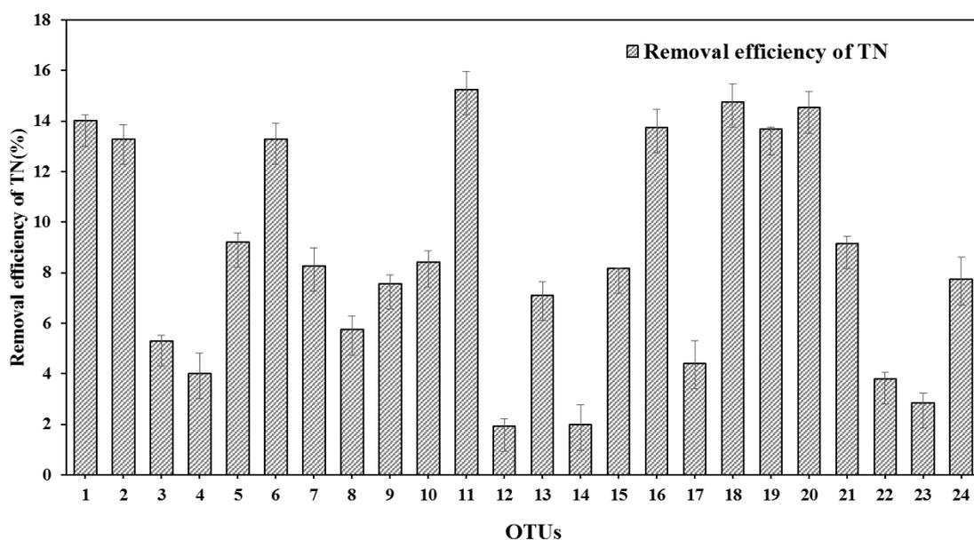
Fig. 10. Denitrification performance of 24 representative strains. TN removal efficiency reflects the heterotrophic nitrifying-aerobic denitrifying capacity.
