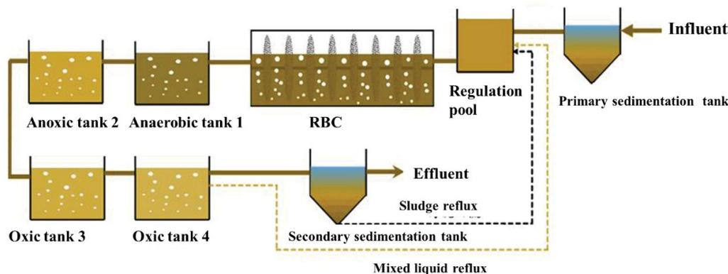
Fig. 1. Process flow diagram of the WWTP system.
