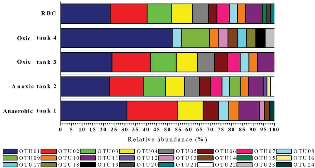
Fig. 8. Relative abundance of aerobic denitrifying bacteria in RBC, anaerobic tank 1, anoxic tank 2, aeration tank 3, and aeration tank 4.
