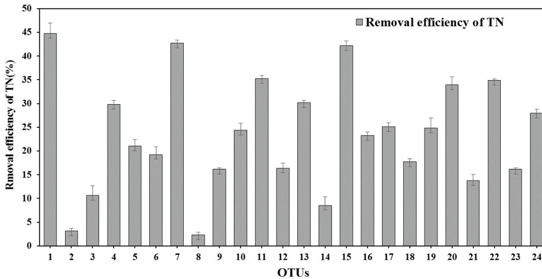
Fig. 9. Aerobic nitrification performance of 24 representative strains. TN removal efficiency reflects the aerobic denitrifying capacity.
