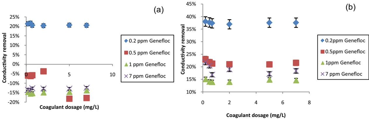
Fig. 9. Conductivity removal with Genefloc as flocculant at (a) 40°C and (b) 60°C.
