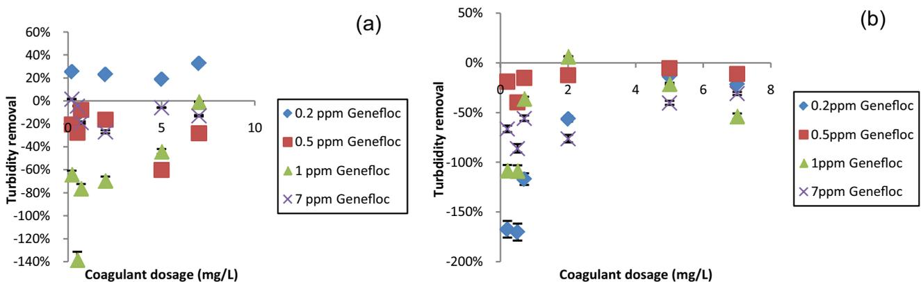
Fig. 10. Turbidity removal with Genefloc as flocculant at (a) 40°C and (b) 60°C.
