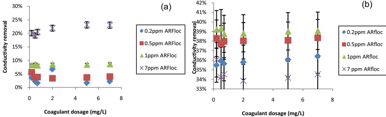
Fig. 5. Conductivity removal with ARFloc100 as flocculant at (a) 40°C and (b) 60°C.
