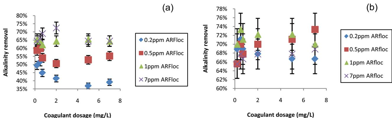
Fig. 8. Alkalinity removal with ARFloc100 as flocculant at (a) 40°C and (b) 60°C.
