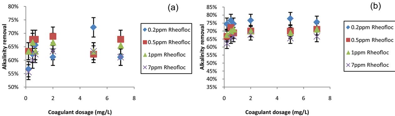
Fig. 4. Alkalinity removal with Rheofloc5414 as flocculant at (a) 40°C and (b) 60°C.
