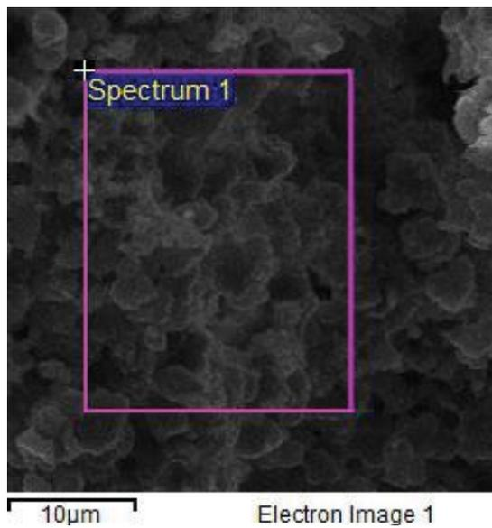
Fig. 14. Electron image of crystals formed using lime with ARFloc100 at 60°C.
