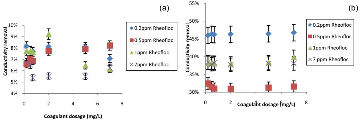
Fig. 1. Conductivity removal with Rheofloc5414 as flocculant at (a) 40°C and (b) 60°C.
