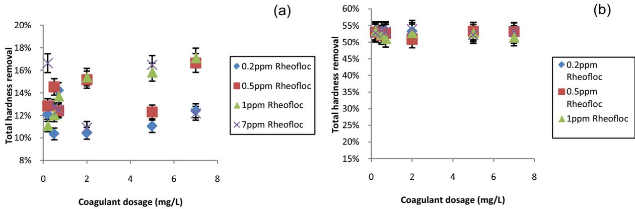
Fig. 3. Total hardness removal with Rheofloc5414 as flocculant at (a) 40°C and (b) 60°C.
