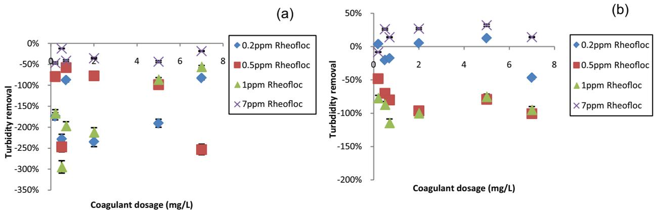
Fig. 2. Turbidity removal with Rheofloc5414 as flocculant at (a) 40°C and (b) 60°C.
