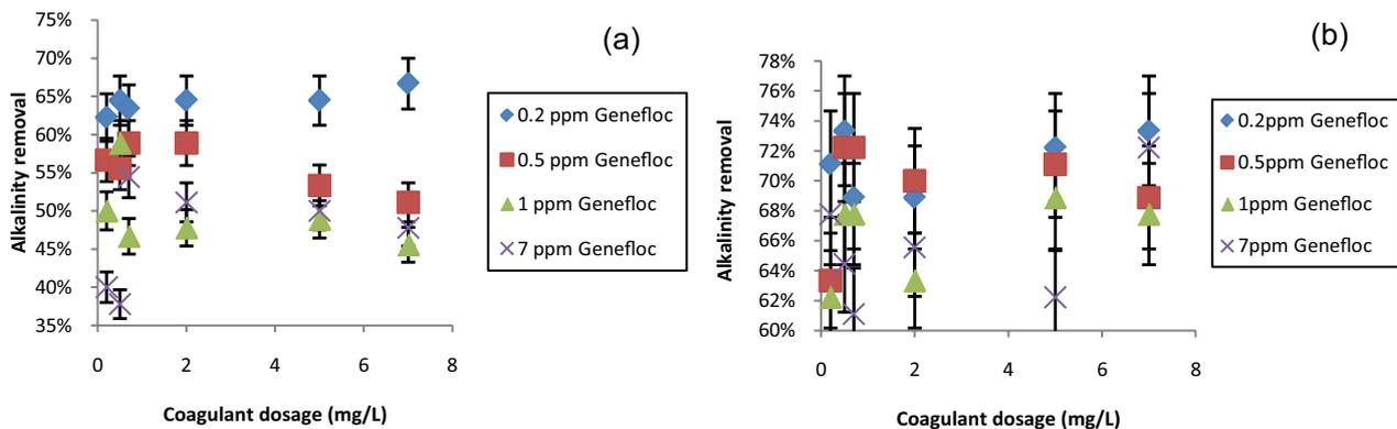
Fig. 12. Alkalinity removal with Genefloc as flocculant at (a) 40°C and (b) 60°C.
