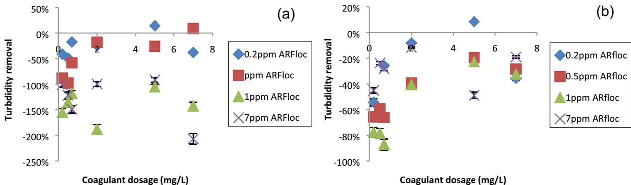
Fig. 6. Turbidity removal with ARFloc100 as flocculant at (a) 40°C and (b) 60°C.
