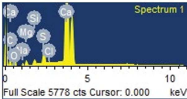
Fig. 17. EMS that illustrates compounds formed when NaOH was used with Rheofloc5414 at 60°C.
