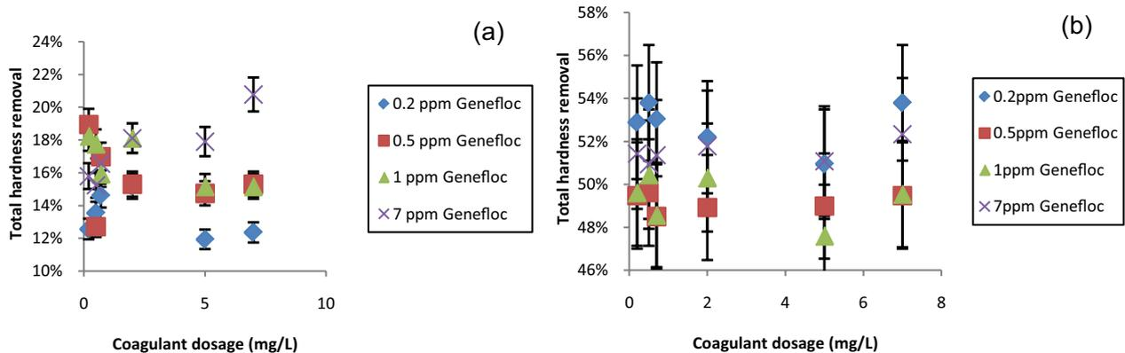
Fig. 11. Total hardness removal with Genefloc as flocculant at (a) 40°C and (b) 60°C.
