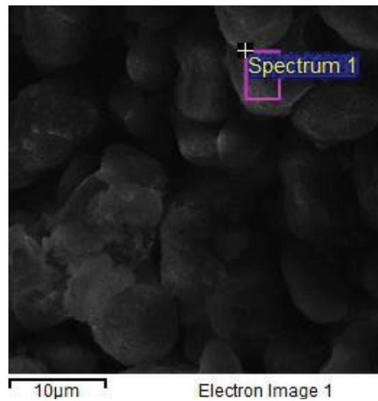
Fig. 16. Electron image of crystals formed using NaOH with Rheofloc5414 at 60°C.
