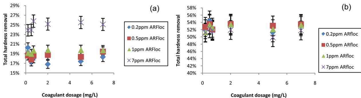
Fig. 7. Total hardness removal with ARFloc100 as flocculant at (a) 40°C and (b) 60°C.
