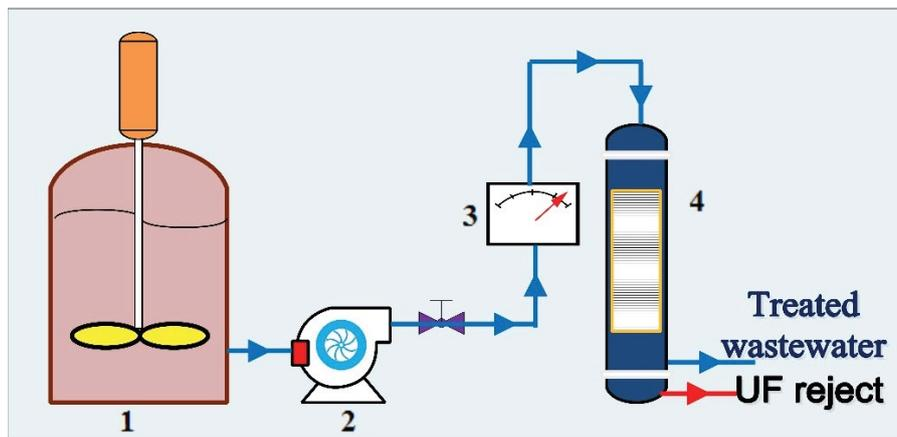
Fig. 3. Schematic of UF set up. (1) Storing tank, (2) peristaltic pump, (3) barometer, and (4) UF module.
