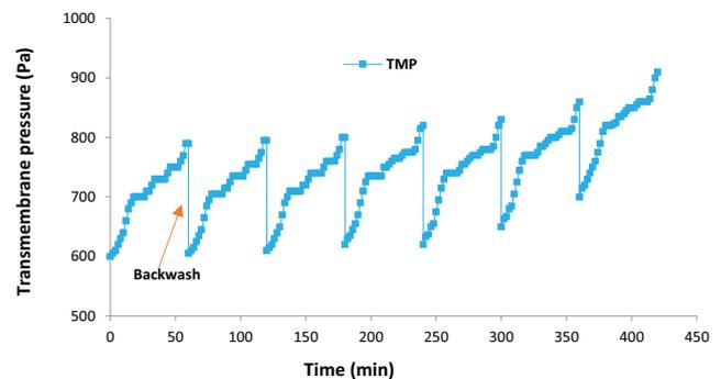
Fig. 7. Variations of TMP during UF system operation.
