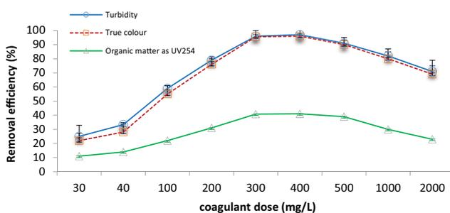
Fig. 6. Variation of CFS process efficiency under coagulant aid and clay addition (solution pH: 7.2, coagulant aid: 2 mg/L, and clay dose: 0.7 g/L).
