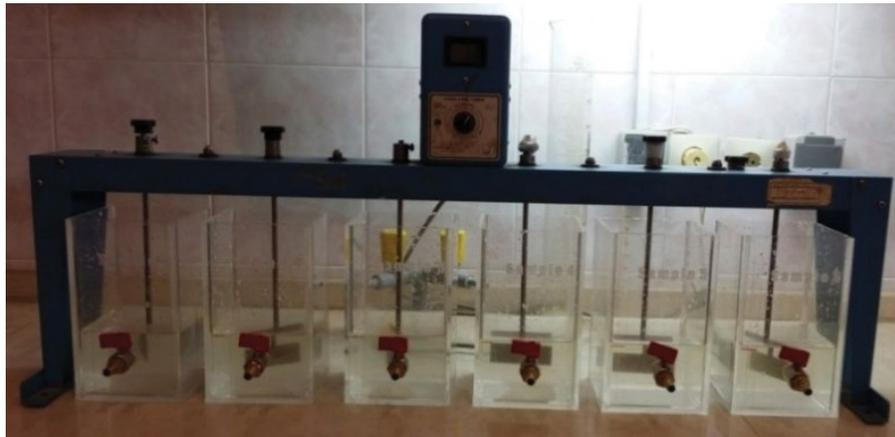
Fig. 2. Photograph of Phipps and Bird jar apparatus.
