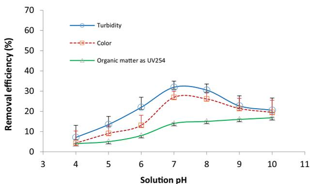
Fig. 4. Effect of solution pH on CFS efficiency (PACl dose: 60 mg/L and coagulant aid dose: 2 mg/L).
