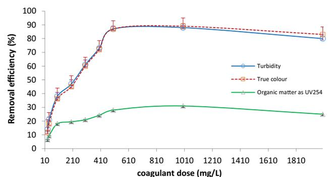
Fig. 5. Variation of removal efficiency of CFS process as a function of coagulant dose (solution pH: 7.2 and coagulant aid dose: 2 mg/L).
