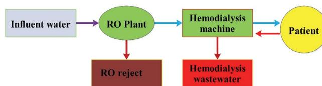
Fig. 1. Diagram of produced wastewater from hemodialysis and RO treatment process.
