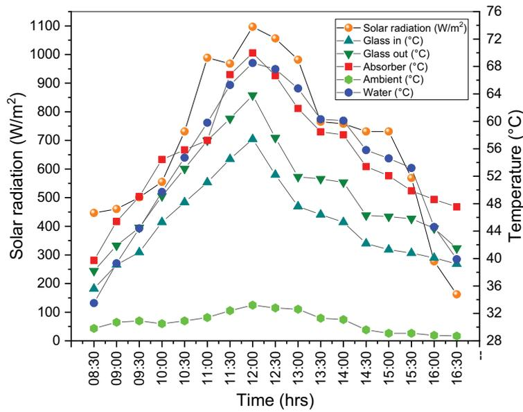
Fig. 9. Variation of solar radiation and different temperatures with respect to time and without ridge gourd.
