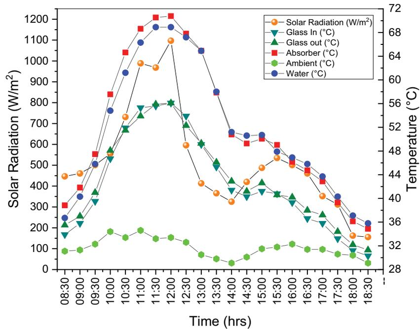
Fig. 6. Variation of solar radiation and different temperatures with respect to time and without ridge gourd.
