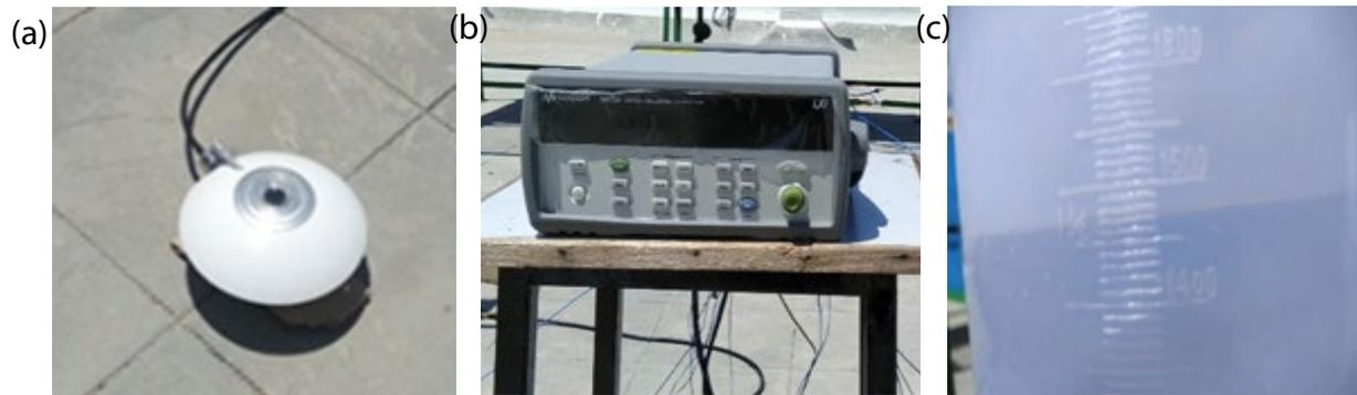
Fig. 2. (a) Pyranometer, (b) data logger, and (c) collecting container.
