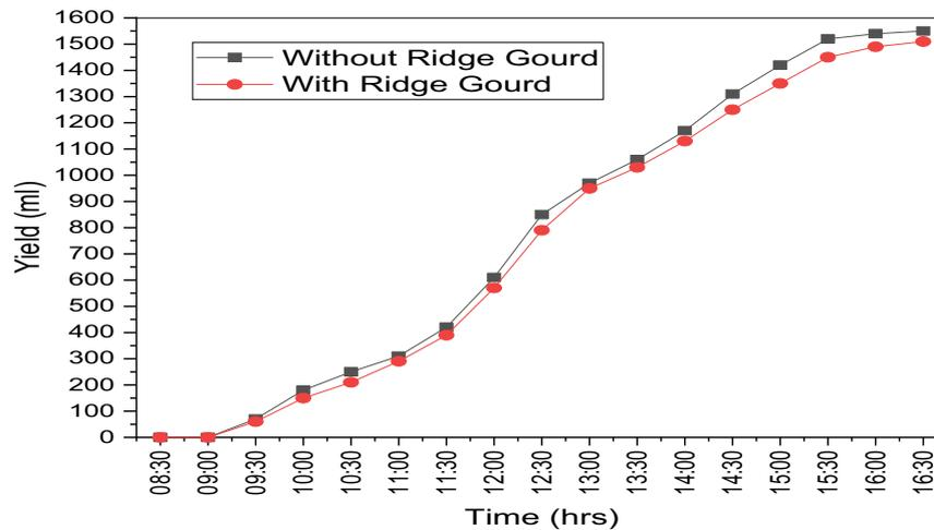
Fig. 11. Variation of distillate yield with respect to time in the desalination setup with and without the inclusion of ridge gourd fiber.
