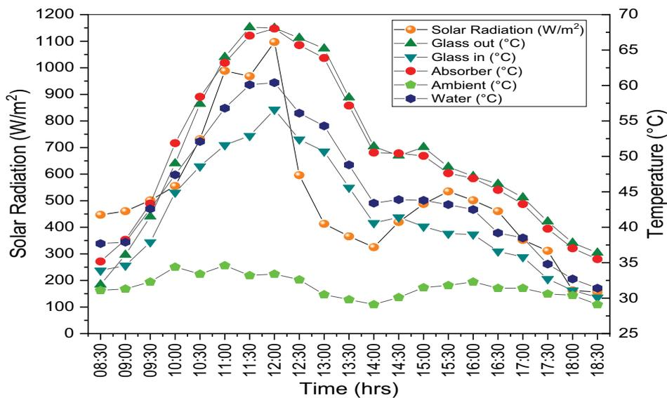
Fig. 7. Variation of solar radiation and different temperatures with respect to time and with ridge gourd.
