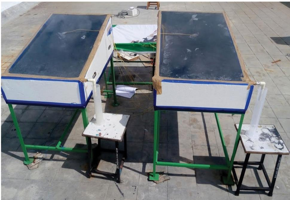
Fig. 1. Single slope solar desalination setup.
