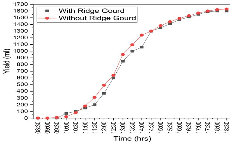
Fig. 8. Variation of distillate yield with respect to time in the desalination setup with and without the inclusion of ridge gourd fiber.
